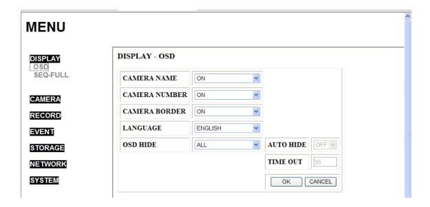
Except setting IP address or web/client ports, every setup of DVR can be made or modified in this page.
