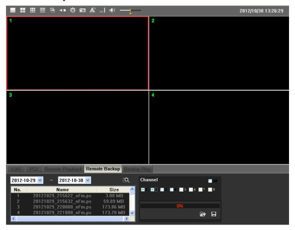
You can archive the recording remotely in this menu. Backup file list is indicated according to selected days and only PS type of files can be archived.
