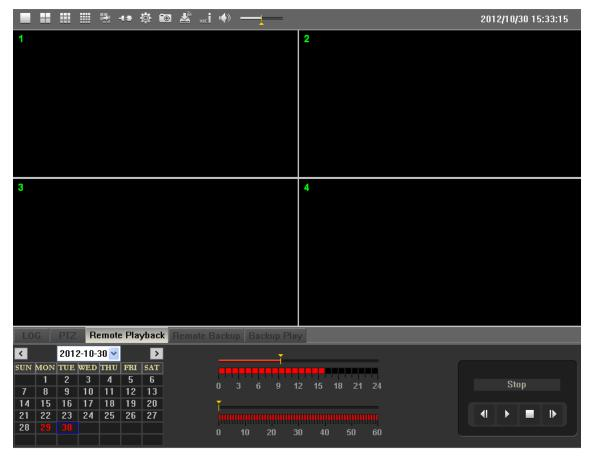
Once you get to "Remote Playback" mode, calendar, time bar & play control buttons are shown at the bottom of screen. On calendar, days with recording are indicated in red color and on time bar as well.
