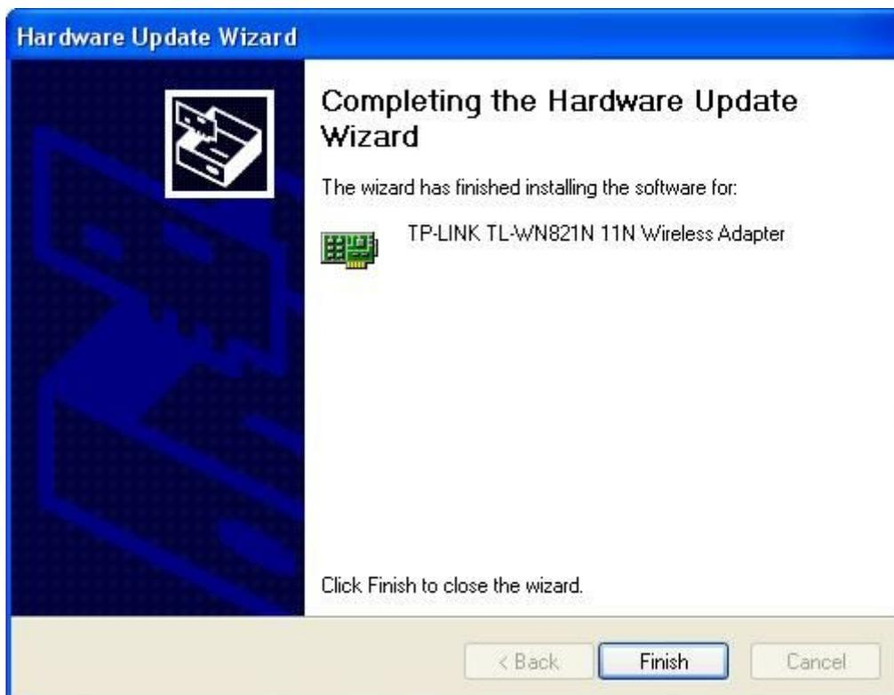
As yet, the adapter has been successfully installed. You can go to **Device Manager** and check **Network Adapters**.
