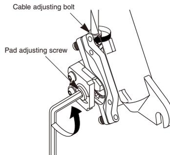
3. Install the new brake pads. After this, bend open the split pin. Tighten the pad adjusting screw so that the clearance between the brake pad and the rotor is 0.2--0.4 mm.
