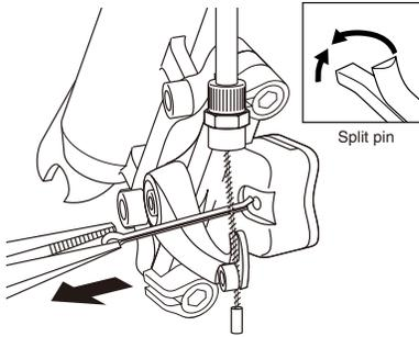
2. Loosen the pad adjusting screw and turn the cable adjusting bolts at the brake lever and caliper body clockwise to loosen them.
