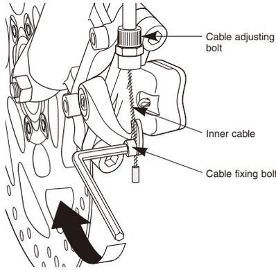
7. Depress the brake lever about 10 times until it touches the grip, and check that there are no problems with any components, and also that the rotors and the pads do not interfere with each other when the wheel is rotated.
