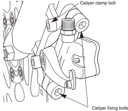
2. While wearing protective gloves, apply pressure to the adapter in the counterclockwise direction while tightening the caliper clamp bolt.
