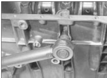
19.12 Tightening No. 3 main bearing side bolt
