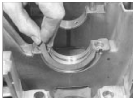
19.3 Fitting thrustwasher upper segments
