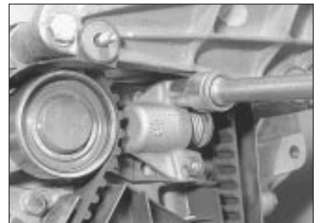
6.12b . . . and tighten drivebelt tensioner front nuts
