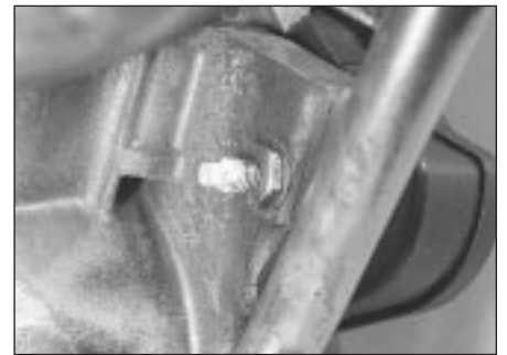
6.8 Tensioner cam spindle (square end) and locknut
