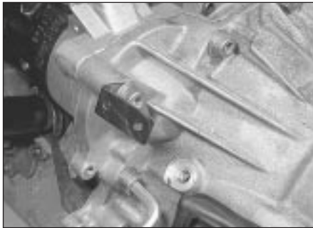
12.1a Starter motor is secured by three Allen bolts . . .
