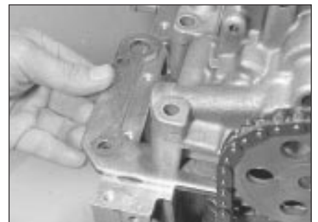
19.19b Locating oil pump spacer
