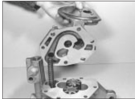
14.10 Separating two halves of oil pump
