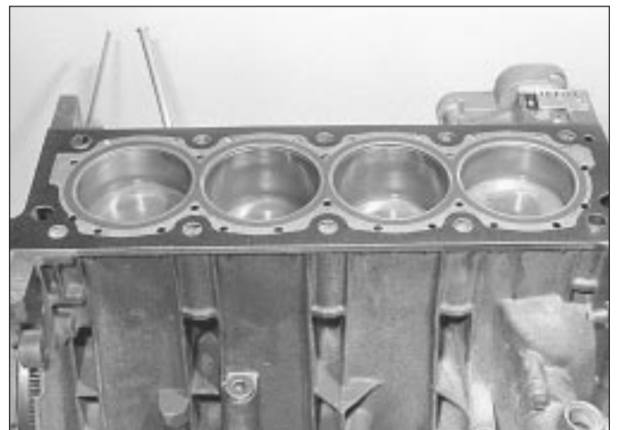
19.28 Head gasket correctly fitted
