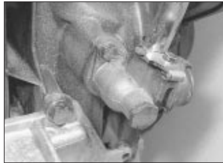
19.49a Securing coolant pipe to inlet housing
