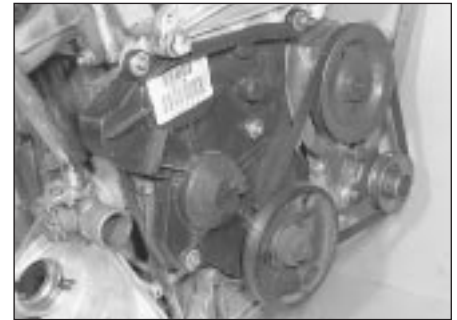
19.49b Refitting HP pump and drivebelt
