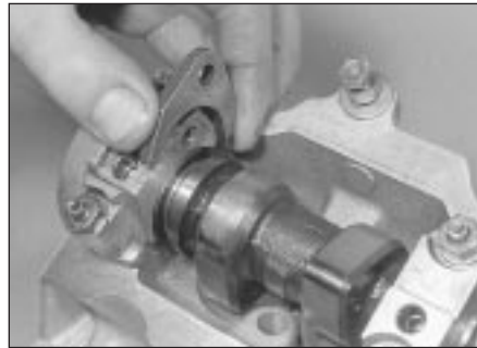
7.7b . . . and remove camshaft thrust plate
