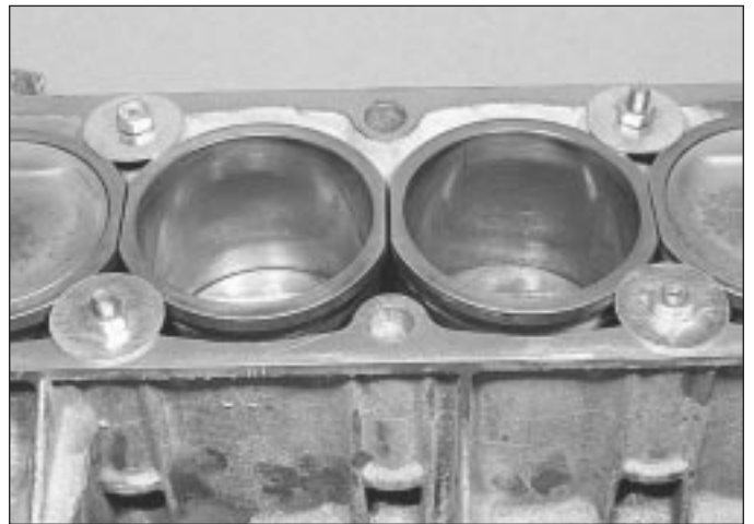
8.20 Cylinder liners clamped with washers and bolts
