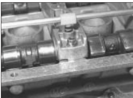
6.33 Camshaft lubrication pipe - note seal on spigot
