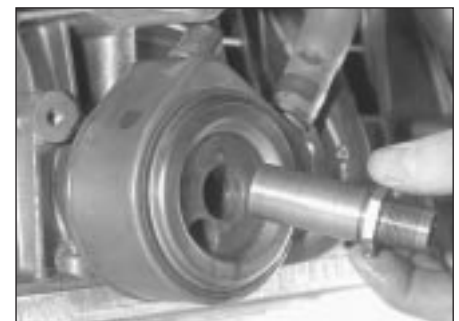
16.32 Fitting oil cooler retaining tube and nut
