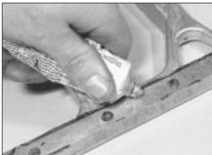
16.18 Applying instant gasket to sump spacer plate
