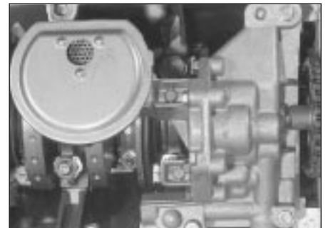
11.34a Oil pump in position
