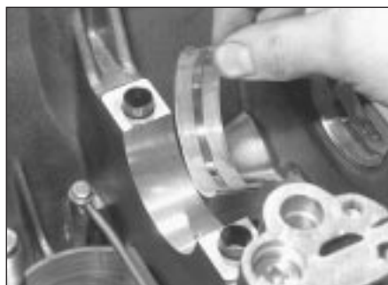
16.2 Fitting a grooved bearing shell to the crankcase
