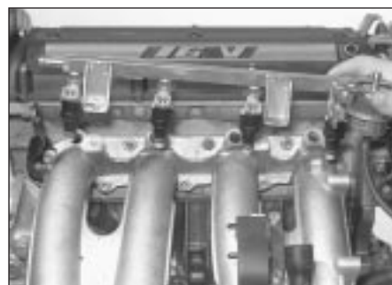
6.41 Fitting fuel rail and injectors
