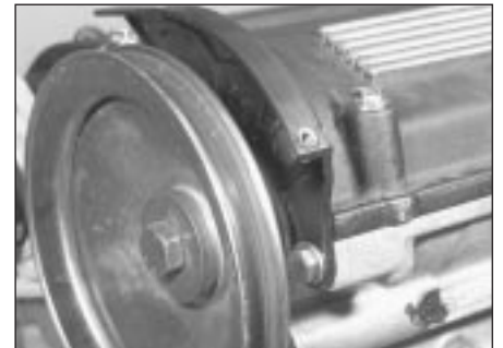
16.36 Camshaft plastic guard and pulley correctly refitted
