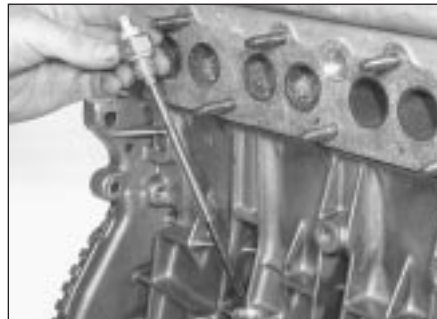
16.35b Refitting oil level sensor
