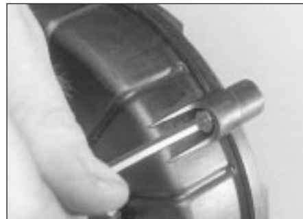
6.8b Extracting a timing belt cover screw
