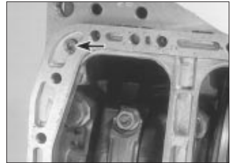
11.32a Extract Allen screws (arrowed) . . .
