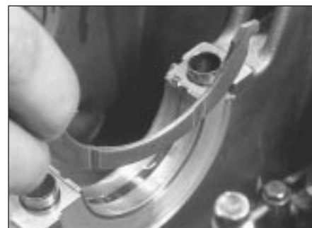
16.3 Fitting a crankshaft thrustwasher
