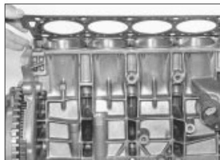
6.28 Fitting a new cylinder head gasket
