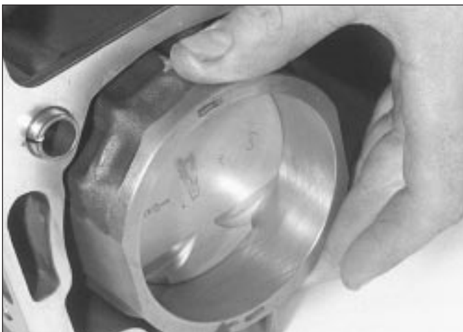
16.12a Fitting a piston/connecting rod/liner assembly
