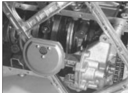
11.32b . . . and remove sump spacer plate
