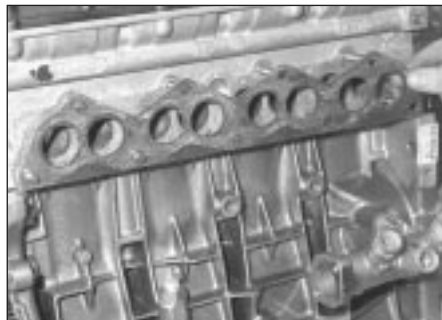
6.38a Exhaust manifold gasket correctly located
