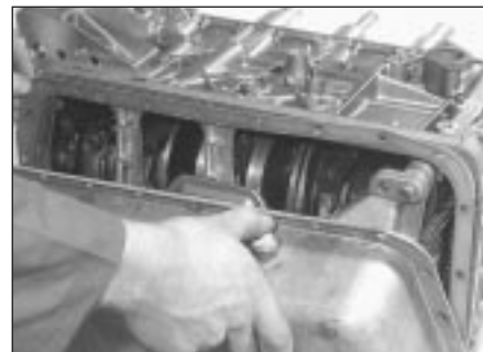
16.19 Refitting sump pan and gasket
