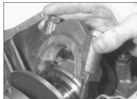
16.5b Fitting a main bearing cap
