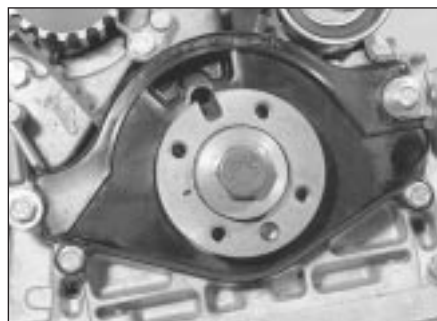
5.18a Timing belt lower cover refitted
