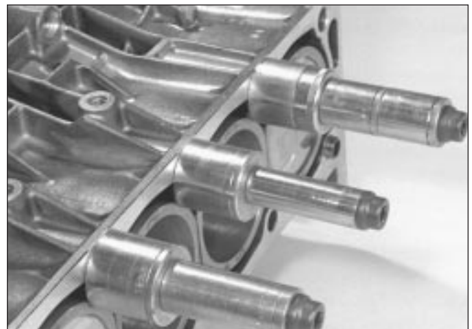
16.12b Typical cylinder liner clamps fitted
