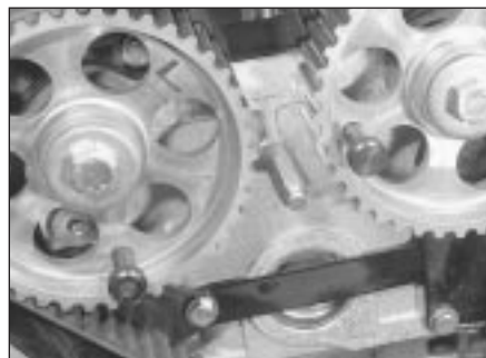
5.12a Camshaft sprocket locking pins in position
