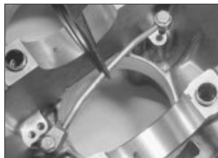
16.1 Fitting a crankcase lubrication pipe
