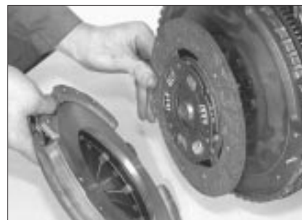
16.21 Fitting clutch components
