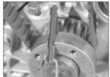
5.12b Crankshaft sprocket locking rod in position
