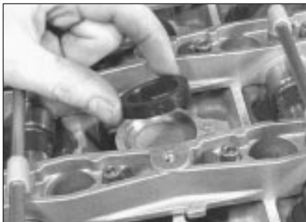
6.36 Spark plug hole oil seal
