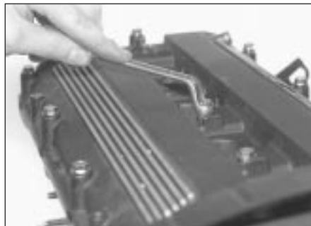
6.8a Extracting a camshaft cover screw
