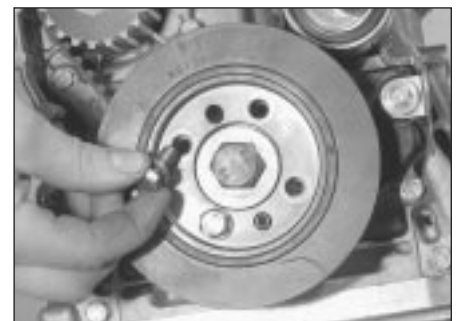
5.18b Fitting a crankshaft damper bolt
