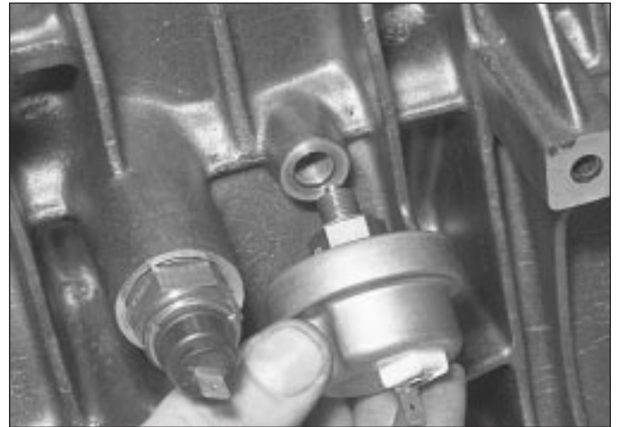
16.35a Refitting oil pressure switch
