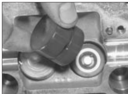
12.4 Removing a hydraulic tappet
