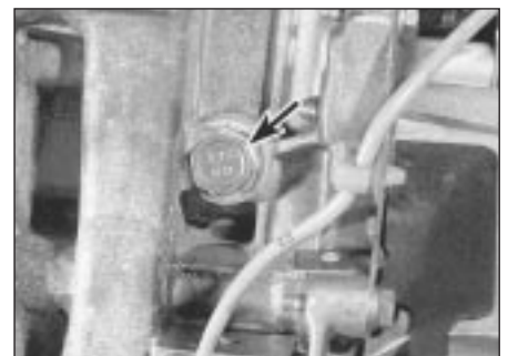
32.4 Cylinder block coolant drain plug - K1G engine
