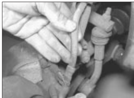
8.4b Examining a brake system hose
