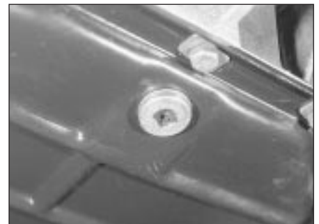
9.3 The engine oil drain plug is located at the lowest point of the sump
