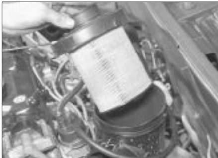
28.5b . . . and withdraw the lid/element assembly - BX 14 with K1G engine
