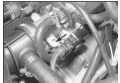
23.9 Idle speed adjustment screw (arrowed) - Bosch LE3 Jetronic
