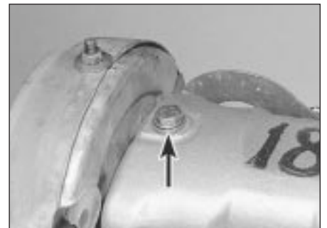
22.9 Copper washer (arrowed) under bolt head
