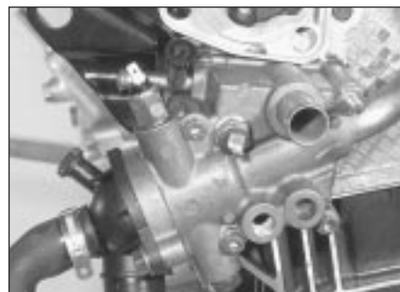
8.1a Thermostat housing in position - BX 19 GTi 16v
