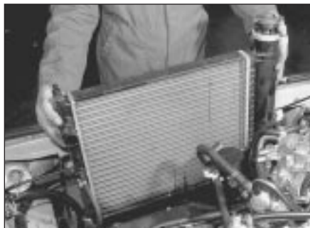
3.5 Lifting radiator out of vehicle
