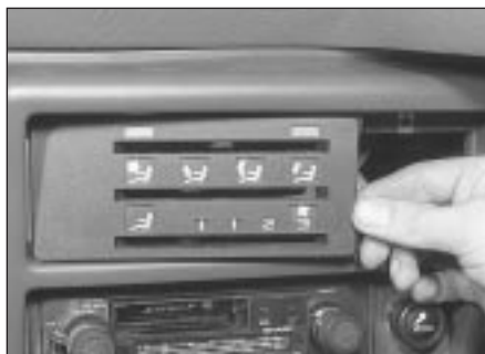
11.8 Heater/ventilation control plate removal
