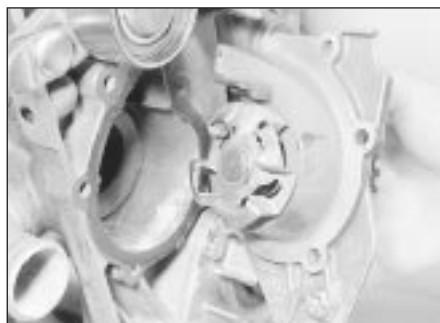
10.12 Coolant pump removal
