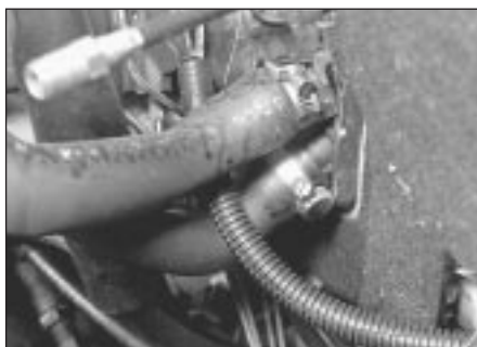
11.21 Heater flow and return hose connections at bulkhead/heater
