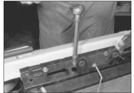
3.4a Undoing radiator retaining bolts
