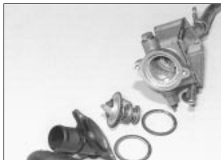
8.1b Thermostat housing dismantled - BX 19 GTi 16v
