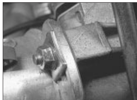
6.6 Distributor timing alignment mark - BX 16
