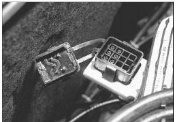
9.1 Diagnostic test socket - BX 16
