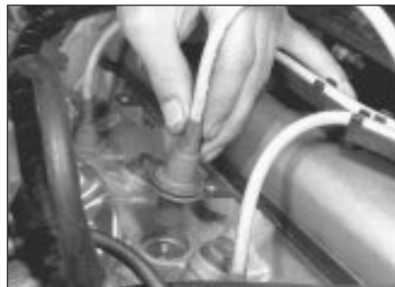
2.2 HT lead removal from spark plug - do not pull on lead
