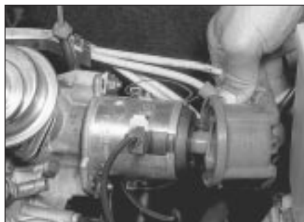
5.3 Removing the distributor cap - BX 16
