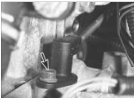
11.3 Crankshaft sensor location (retaining screw arrowed)
