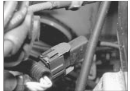
11.2 Crankshaft sensor wiring connector situated behind ignition coil
