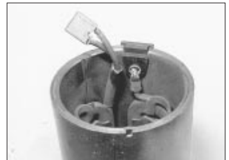
10.7 Brush connections to field coil
