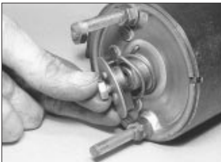
10.3 Removing seal assembly and spring
