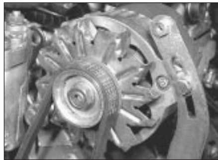
5.2 Alternator drivebelt and adjustment strap - BX 16
