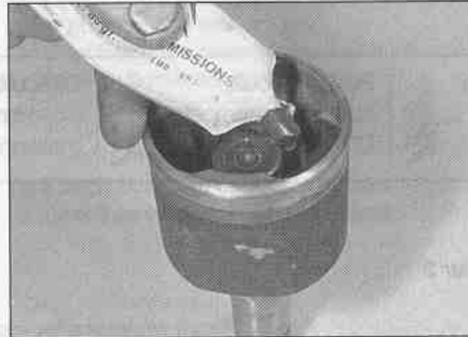
2.11 Injecting grease into the inner joint housing
