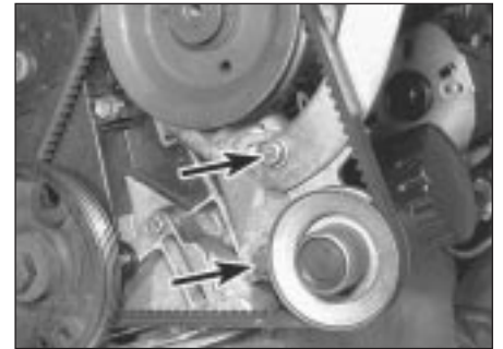
6.2 HP pump drivebelt jockey wheel mounting and adjuster bolts (arrowed) - BX 16
