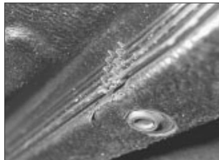
3.3a Hydraulic pipes and retaining clips which keep them correctly located
