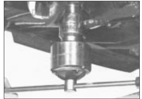
15.7 Balljoint unit removal using recommended impact wrench
