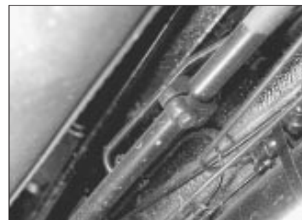
10.5 Rear anti-roll bar and height corrector clamp
