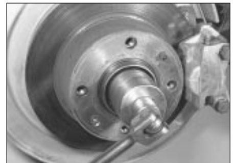
7.1b . . . and loosen the hub nut
