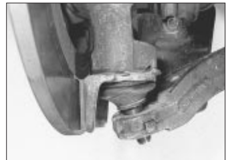
3.10 Separate swivel balljoint from suspension arm
