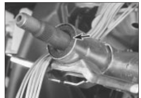
16.17 Upper steering column oil seal (arrowed)
