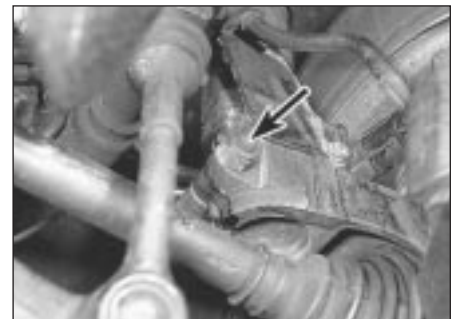
5.8 Swivel hub-to-suspension unit clamp bolt (arrowed)
