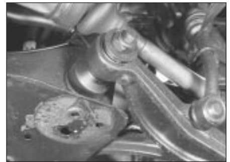
3.1b Later type of front suspension arm and subframe
