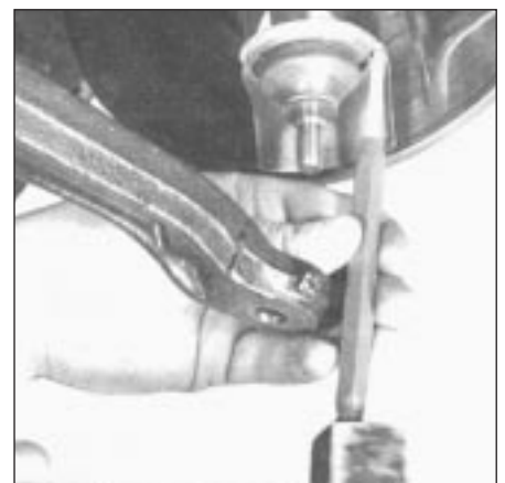
15.8c Carefully drive protector plate into position
