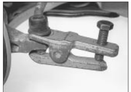
13.2b . . . and use a separator to detach the joint
