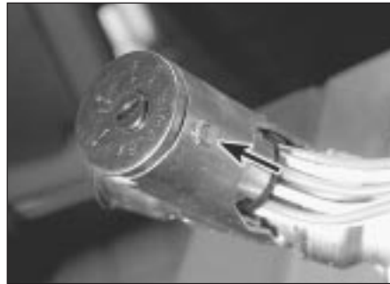
18.4 Remove the bolt (arrowed) . . .
