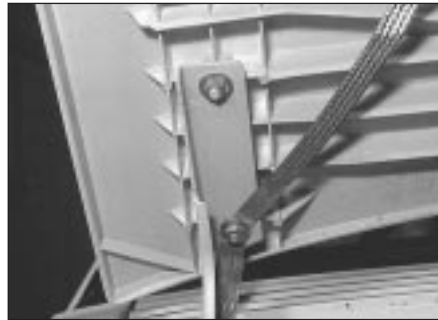
6.3 Bonnet hinge retaining nuts. Note earth strap under lower nut and washer
