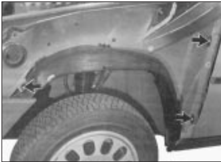
8.9 Captive nut locations (arrowed) for attachment of front wing
