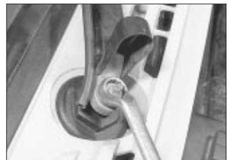
18.3 . . . and unscrew the wiper arm retaining nut
