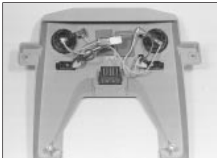
4.4b Map reading light/ sunroof console removed
