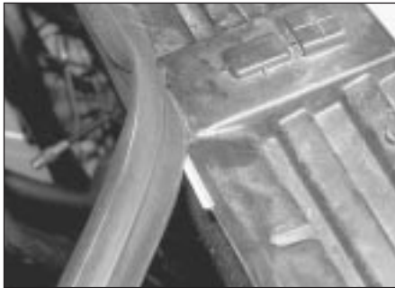
19.3a Peel back the cover seal . . .
