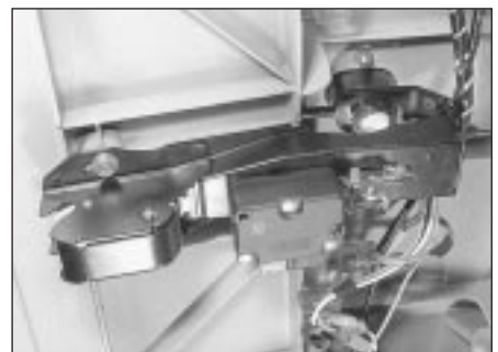
25.10 Tailgate central locking solenoid and lock unit
