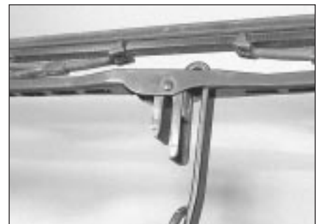
17.2 Wiper blade removal from arm
