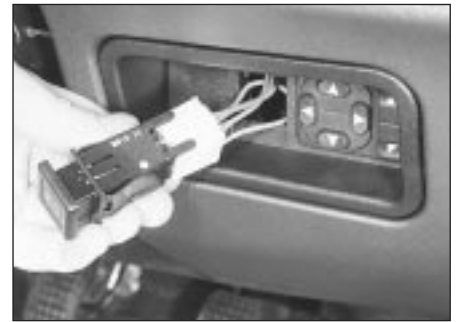
12.4 Refitting the front foglight switch
