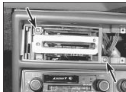
28.4 Remove the panel screws indicated
