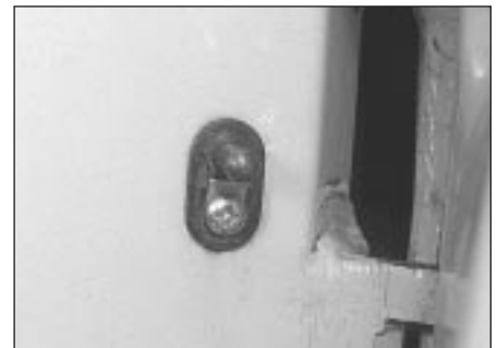
10.2 Door courtesy light switch retaining screw
