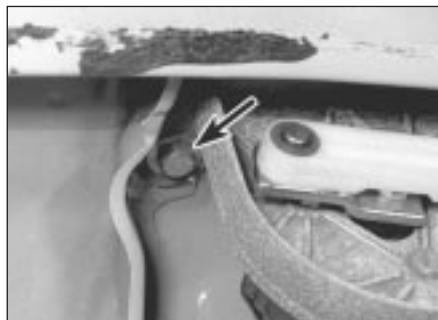
19.6a Wiper motor retaining bolt (arrowed)
