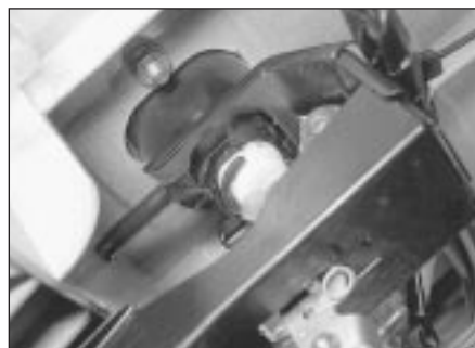
25.9 Lock barrel and retaining clip (central locking)
