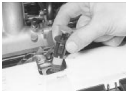
26.4 Removing the bonnet-open warning switch
