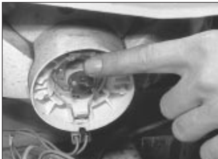
3.4 Align the headlamp bulb
