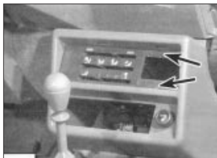
28.3 Ashtray holder/heater control plate retaining screws (arrowed)
