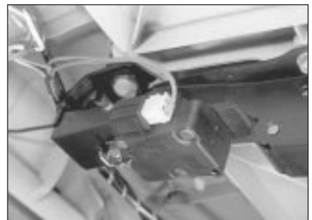
25.8 Wiring connector to the tailgate solenoid (central locking)
