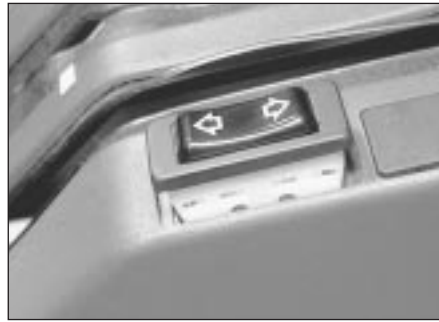
11.2 Electric window operating switch removal
