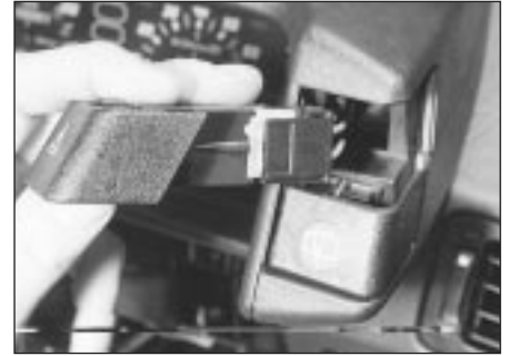
8.2 Removing a facia switch
