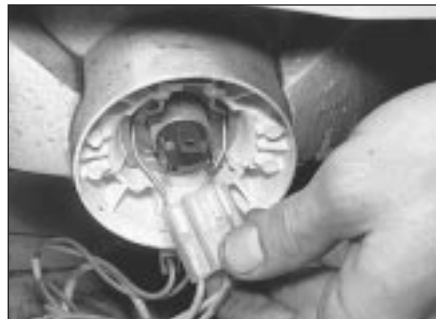
3.2a Disconnect the wiring connector . . .
