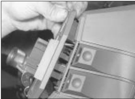
9.5 Withdrawing the multi-connector panel
