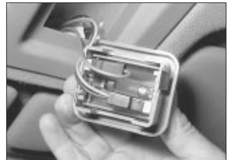
4.6 Interior map lamp bulb - festoon type
