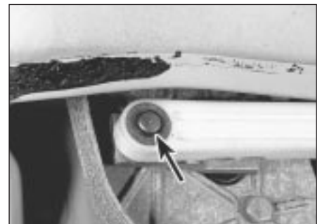
19.6b Wiper motor linkage arm spring clip (arrowed)
