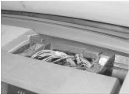
7.3 Remove the instrument panel upper fixing screws (arrowed)
