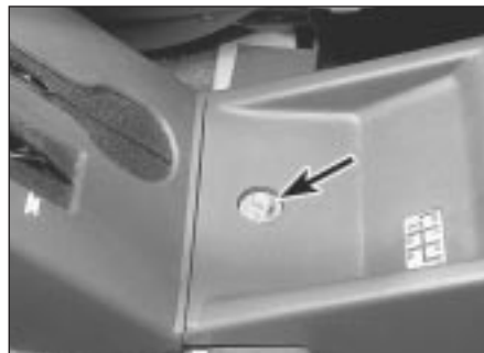
13.3 Console retaining bolt (arrowed)
