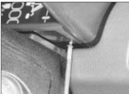
7.12 Unscrewing a trim panel retaining screw
