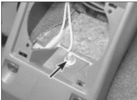
13.2 Handbrake console retaining nut (arrowed)
