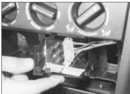
26.3 Removing the door warning panel
