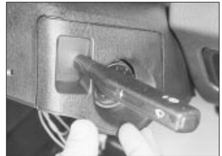
9.13b Removing the steering column upper shroud side panel
