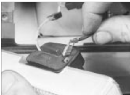
3.10 Disconnecting the foglight wiring
