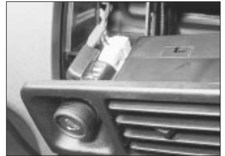
14.8 Withdrawing the grille panel
