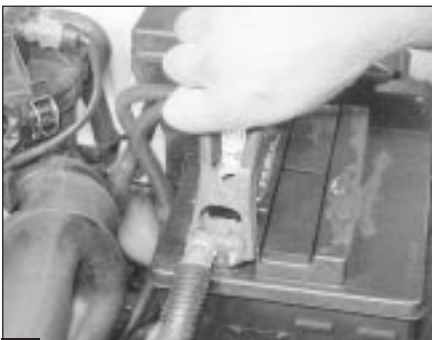
1 Connect one end of the red jump lead to the positive (+) terminal of the flat battery
