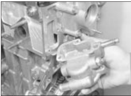
7.17 Removing thermostat housing
