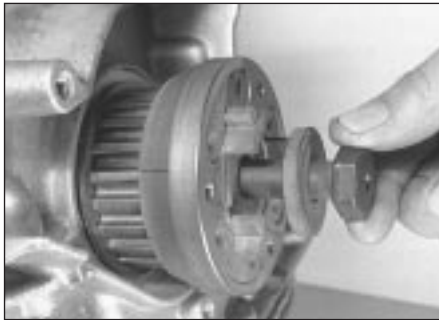
12.34a Removing crankshaft sprocket bolt . . .
