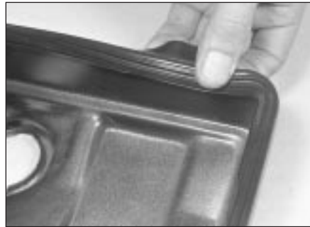
6.3b Removing rocker cover gasket
