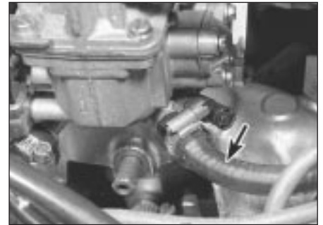
8.26 Heater hose connection at carburettor (arrowed)
