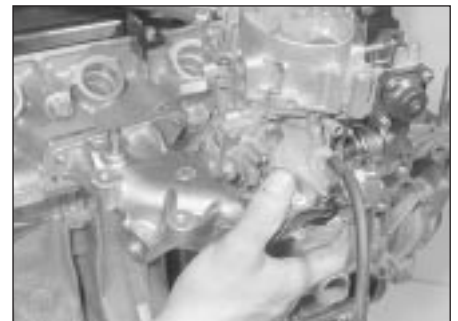
7.9 Removing inlet manifold complete with carburettor
