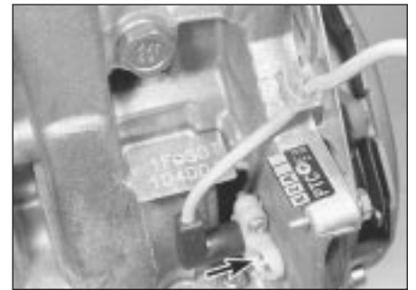
7.19 TDC sensor mounting bolt (arrowed)
