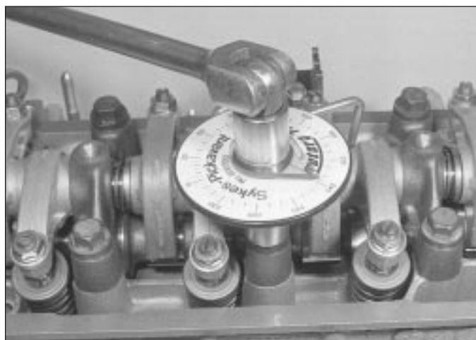
7.41 Angle-tightening cylinder head bolts
