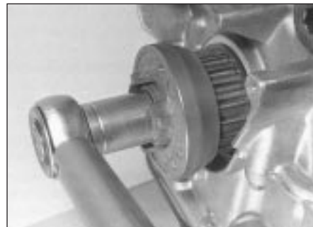
18.28 Tightening crankshaft sprocket bolt
