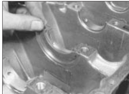
12.51b ... and endfloat thrustwasher
