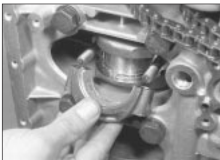
12.44 Removing a big-end bearing cap
