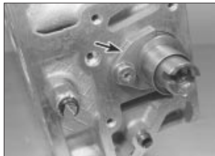
14.2 Camshaft thrust fork (arrowed)
