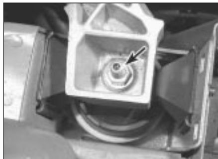
8.31 Right-hand engine mounting through-bolt (arrowed)
