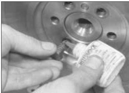
18.25 Applying locking fluid to a flywheel bolt
