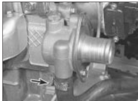
7.8 Water pump hose (arrowed) at thermostat housing
