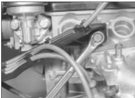
7.6 Unbolting HT lead support
