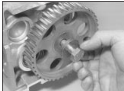
14.1b Unscrew camshaft sprocket bolt ...
