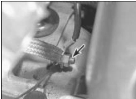
8.27 Earth cables at transmission (arrowed)
