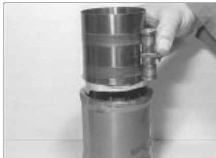
18.14a Fitting a piston ring compressor
