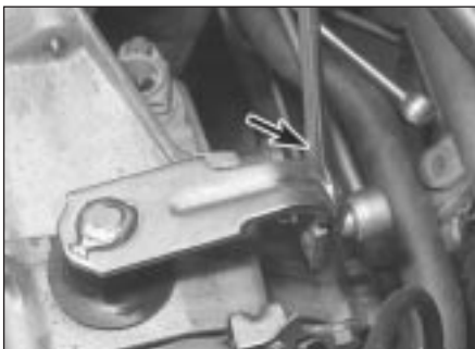
8.15 Using an open-ended spanner (arrowed) to disconnect a gearchange rod balljoint
