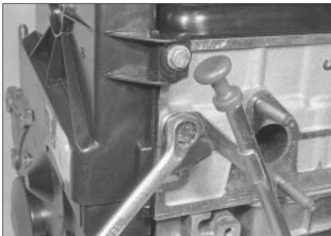
12.18 Unbolting dipstick holder upper mounting
