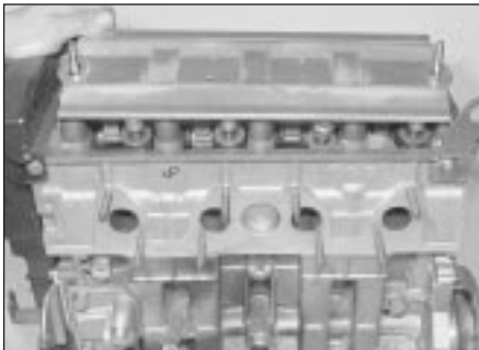
6.4b . . . and baffle plate
