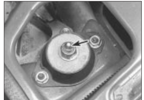
8.30a Left-hand engine mounting through-bolt (arrowed)
