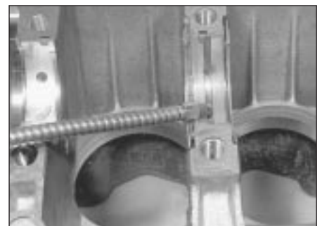
18.3 Oiling main bearing shells
