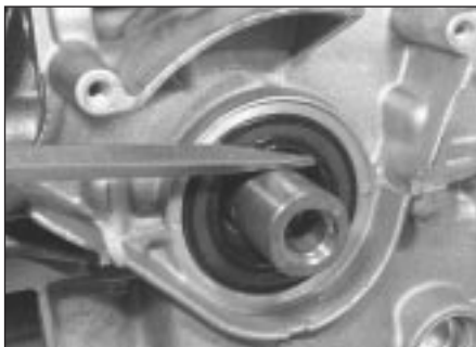
12.35 Prising out crankshaft front oil seal
