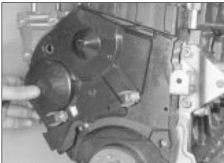
6.5c Removing intermediate timing cover
