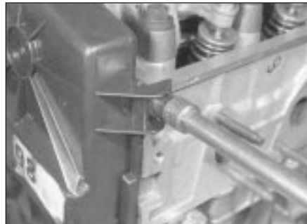
6.5a Unbolting upper timing cover
