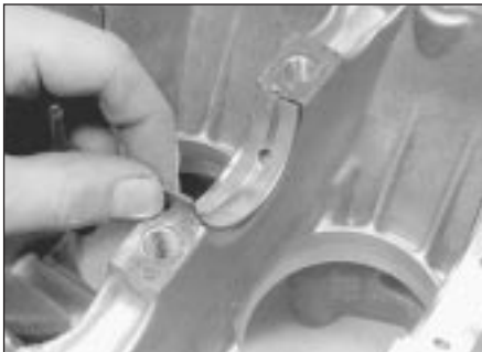
12.51a Removing a main bearing shell ...
