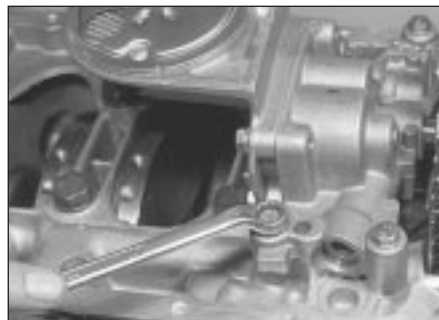
12.40a Unscrew oil pump retaining bolts . . .
