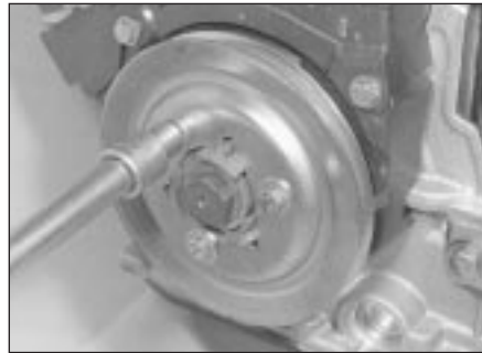
7.12 Unbolting crankshaft pulley
