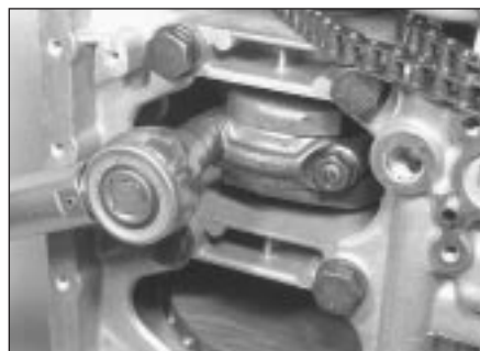
18.17 Tightening a big-end bearing cap nut
