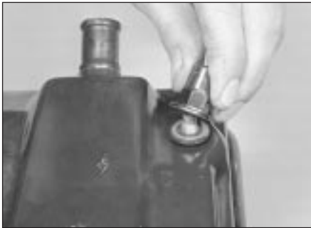
6.3a Removing a rocker cover nut
