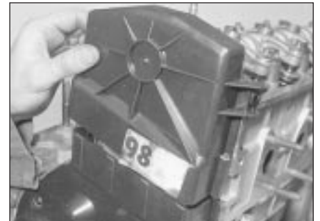
6.5b Removing upper timing cover
