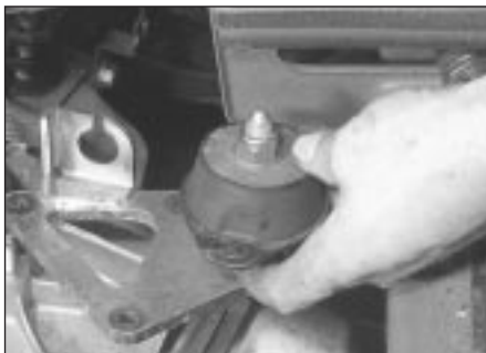
8.30b Removing left-hand engine mounting bracket
