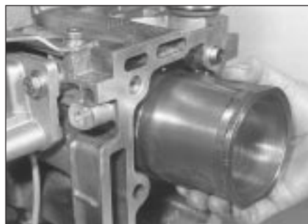
12.45 Removing a liner/piston assembly
