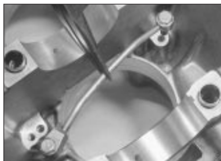
16.1 Fitting a crankcase lubrication pipe
