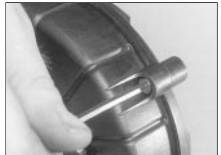
6.8b Extracting a timing belt cover screw
