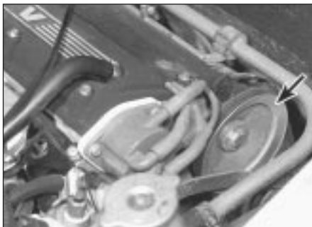
7.3a Hydraulic pump drive pulley (arrowed)
