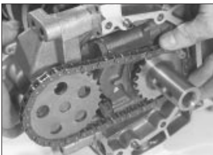
11.34b Removing oil pump with drivechain and sprocket
