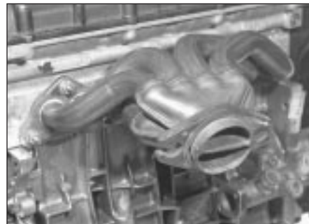
6.38b Exhaust manifold fitted
