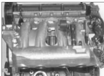
6.38c Inlet manifold fitted
