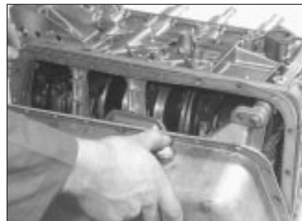
16.19 Refitting sump pan and gasket
