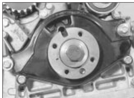
5.18a Timing belt lower cover refitted
