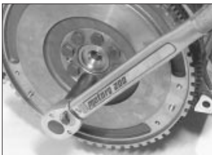
16.20 Tightening a flywheel bolt
