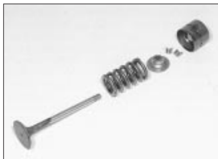
6.23b Valve components
