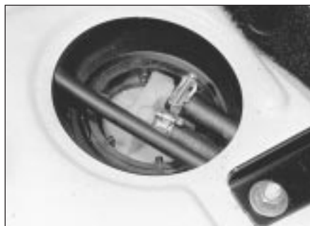
7.2 Fuel tank supply and return hoses - GTi
