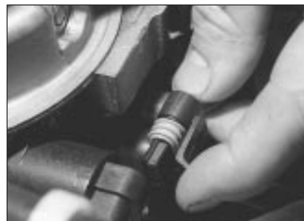
12.2b . . . the idle control stepper motor . . .
