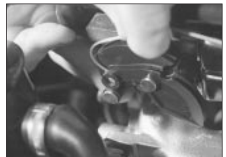
12.4 Disconnecting accelerator inner cable from throttle cam
