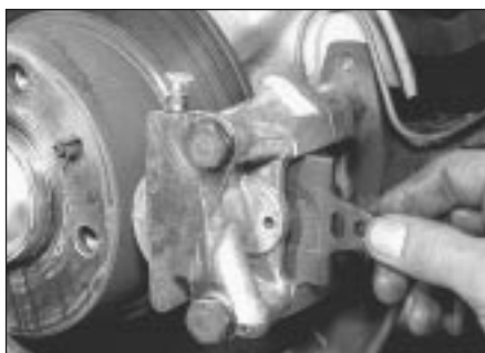
2.19b ... to extract brake outer pad ...
