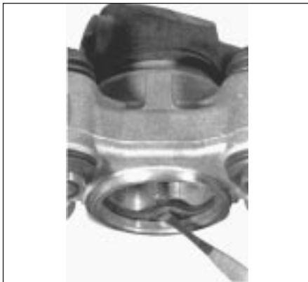
4.15 Prise free the cylinder inner seal
