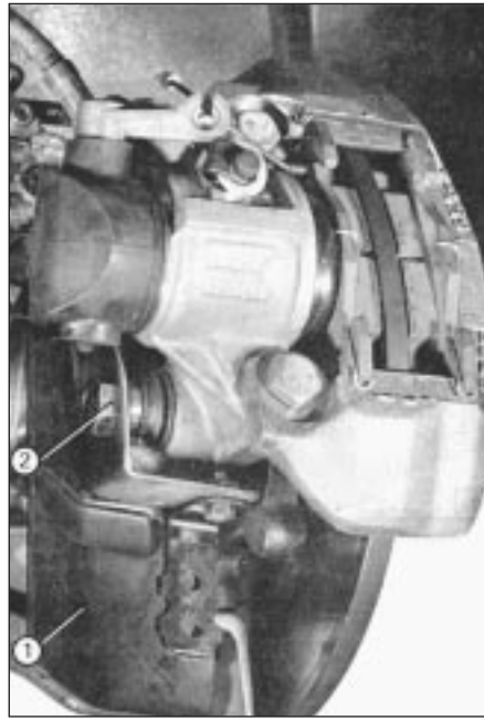
4.8 Front brake caliper deflector (1) and retaining bolt (2)
