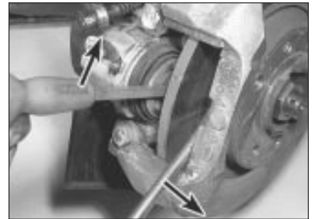
2.7 Method used to move caliper piston back into cylinder
