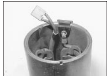
10.7 Brush connections to field coil
