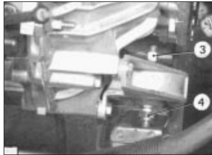
9.5 Remove the engine mounting nuts 3 and 4
