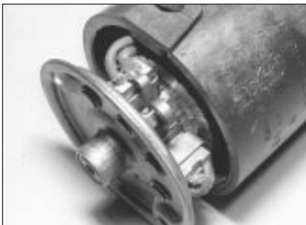
10.4 Removing bearing plate
