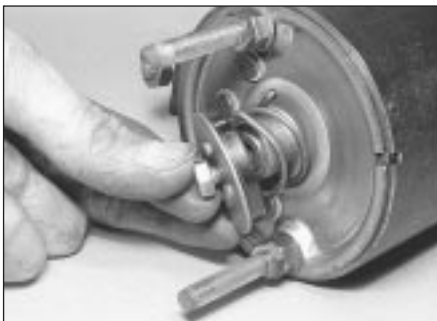
10.3 Removing seal assembly and spring
