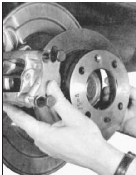
3.9 Rear brake disc removal
