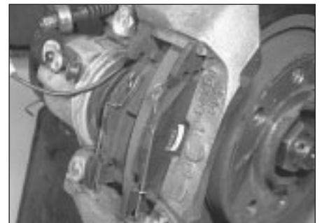
2.11b Brake pads and springs fitted
