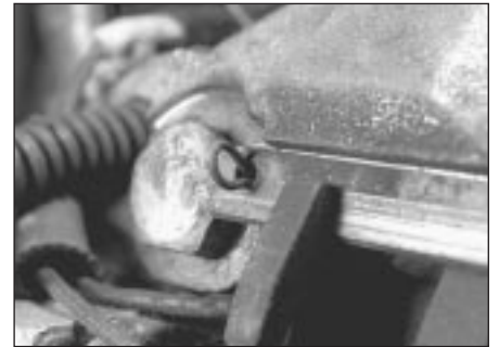
2.5a Extract the lock plate pin . . .
