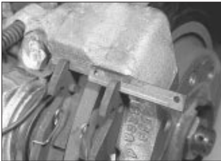
2.5b . . . and withdraw the lock plate
