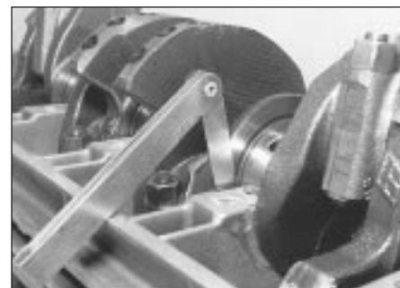
17.17 Checking crankshaft endfloat
