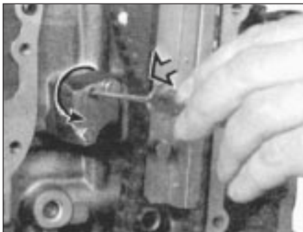
11.3a Loosening first type chain tensioner
