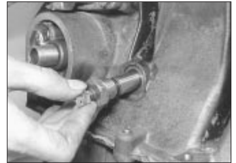
17.41 Oil pressure sender switch
