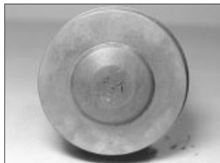
17.6 Piston crown showing directional arrow
