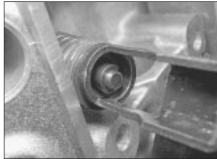
13.2 Compress valve spring ...
