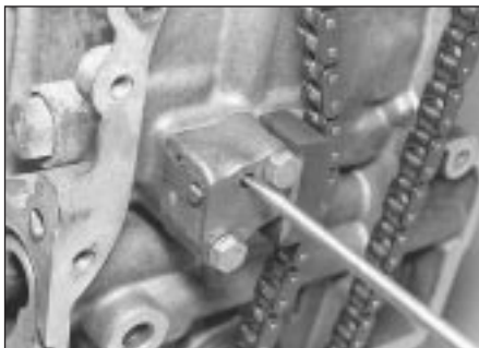
17.36 Releasing timing chain tensioner - first type
