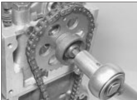
17.35b Tightening sprocket retaining bolt
