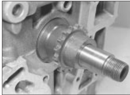
17.32 Locate crankshaft sprocket
