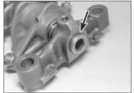
12.34a Rocker shaft retaining circlip (arrowed)
