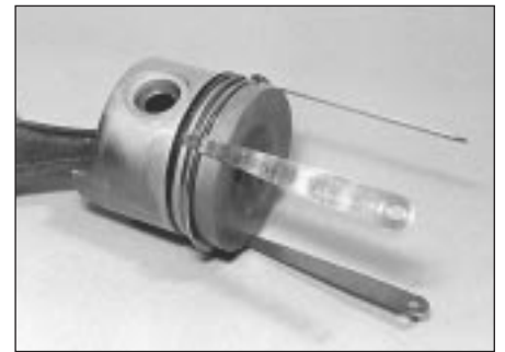
17.1 Method of fitting piston rings
