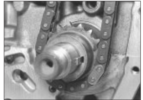
17.33 Timing chain bright link at crankshaft sprocket
