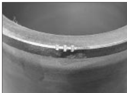
17.4 Piston/liner grading mark
