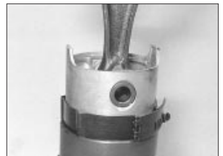
17.8 Fitting the piston/rod assembly to its cylinder liner
