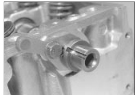
13.1a Remove camshaft retaining plate . . .
