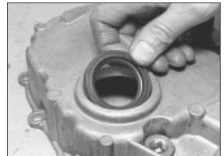
12.29 Renewing timing cover oil seal
