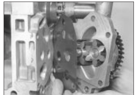
17.39 Fitting oil pump with spacer plate
