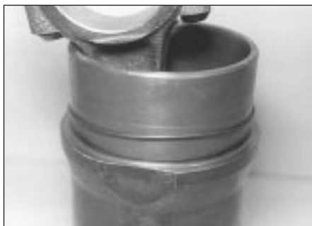
17.10 Cylinder liner O-ring seal
