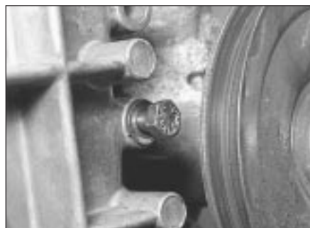
18.8b Timing cover bolt nearest coolant pump pulley
