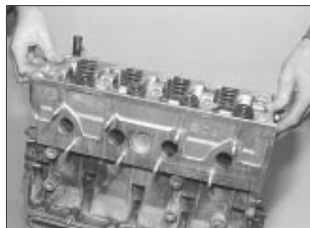
6.34a Lower cylinder head into position . . .
