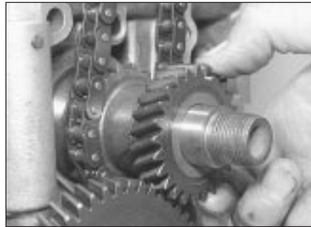
17.40 Oil pump drive sprocket
