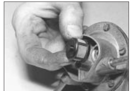
6.2 Fuel pump filter removal
