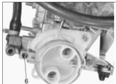
13.5a Solex 32-34 - mixture adjustment screw location (6)
