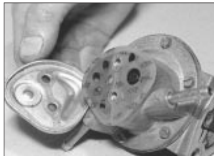
6.1b Fuel pump cover removal - removable filter type
