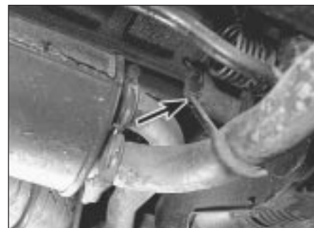
26.3 Exhaust system flexible hanger (arrowed)
