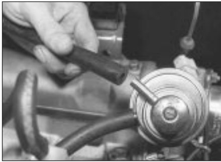
7.1 Fuel supply hose removal from fuel pump
