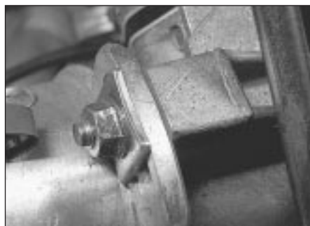
6.6 Distributor timing alignment mark - BX 16
