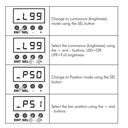
Note: although the unit displays 0-99, there are some finer settings in between each full number, so the number will not change every time you press the button.
