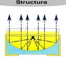
The light from LED is reflected by the reflective mirror inside of the package and radiated outside as the parallel beam.
