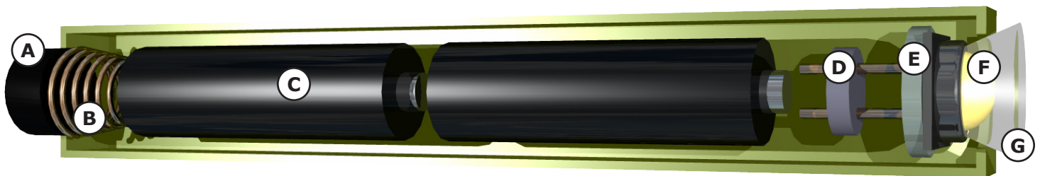
A: ON/OFF Switch, B: Mechanical Spring, C: Battery, D: Driver, E: PCB/Thermal, F: LED, G: Secondary Optic
