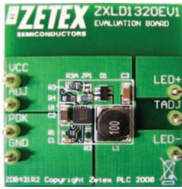
ZXLD1320EV1 evaluation board – a buck LED driver easily configured to drive up to four external LEDs at 1A or 1.5A, housed in the 3 mm x 4 mm TDFN1443 package
