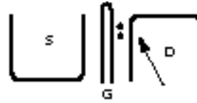
Figure 2. Typical Location of ESD damage in FETs
