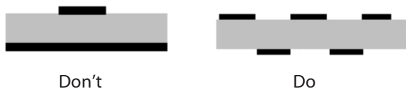
Figure 2. Example of copper spreading on flex
