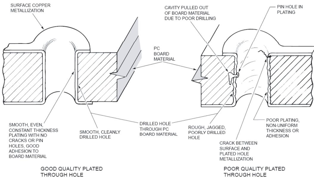
**Figure 9. Attributes of good and poor quality plated through hole**
