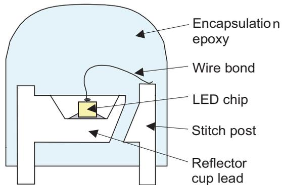
Figure 3. Common TH LED construction
