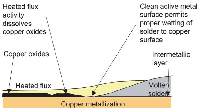
The flux heated to temperature, dissolves the copper oxides leaving a clean, chemically active copper surface and prevents further oxidation. The molten solder immediately wets the copper surface.
