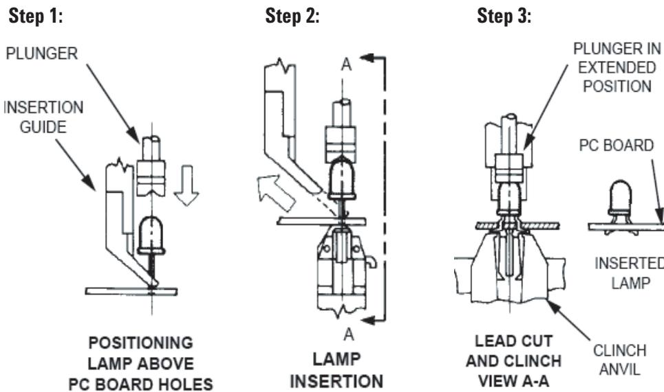
Figure 10. Example of auto-insertion of LED components
