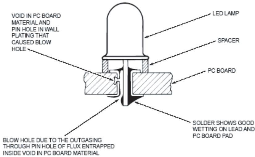
**Figure 8. Typical characteristics of a blow hole defect in a through hole solder connection**
