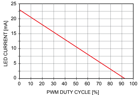
Figure 3. Filtered PWM Dimming [0V to 2.5V]
