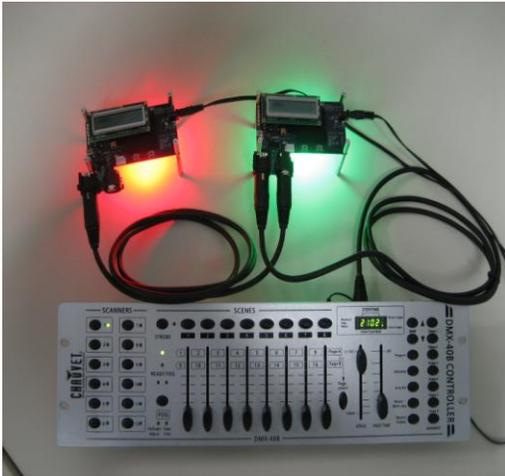
Figure 13. CY3261A RGB Evaluation Kit with RS485 Interface Board
