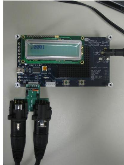
Figure 14. Schematic of Interface Circuit between DMX Controller and EZ-Color Device
