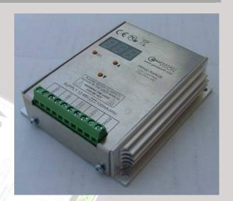
The PP500/PP520 Range has options for normal or fast pulsing and with or without Ethernet interface.
