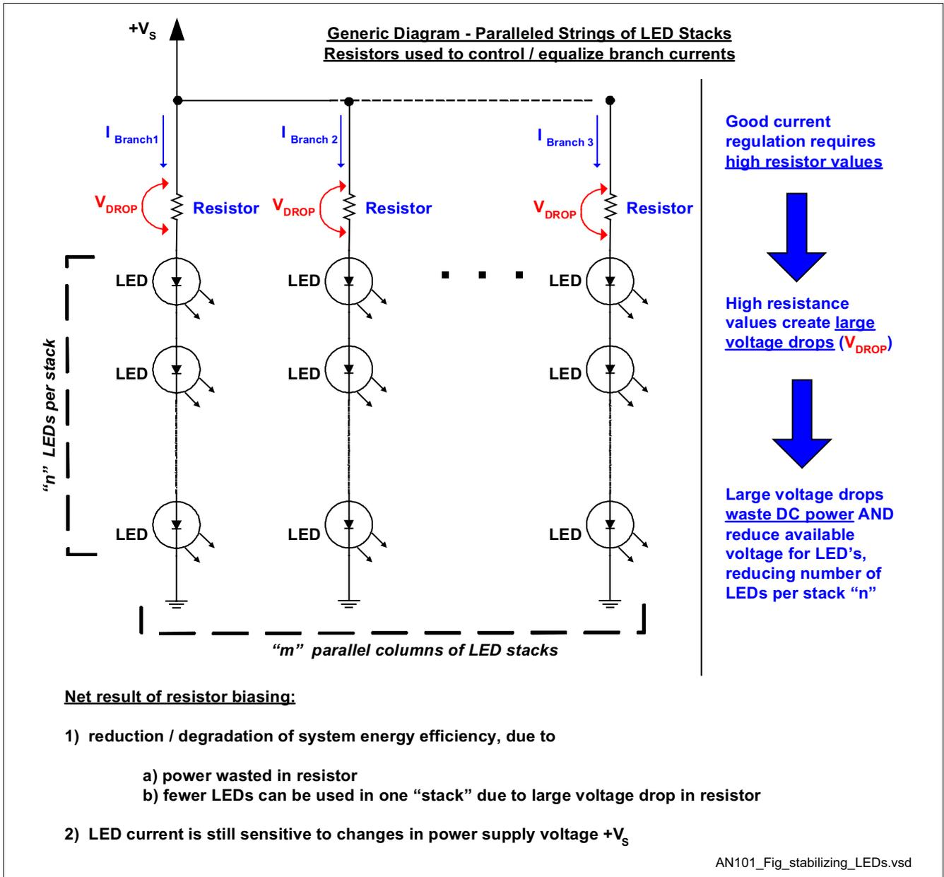
**Figure 3 Resistors used to stabilize / equalize LED operating current for multi-branch LED array, with "n" LEDs per stack and "m" parallel stacks or columns of LEDs**
