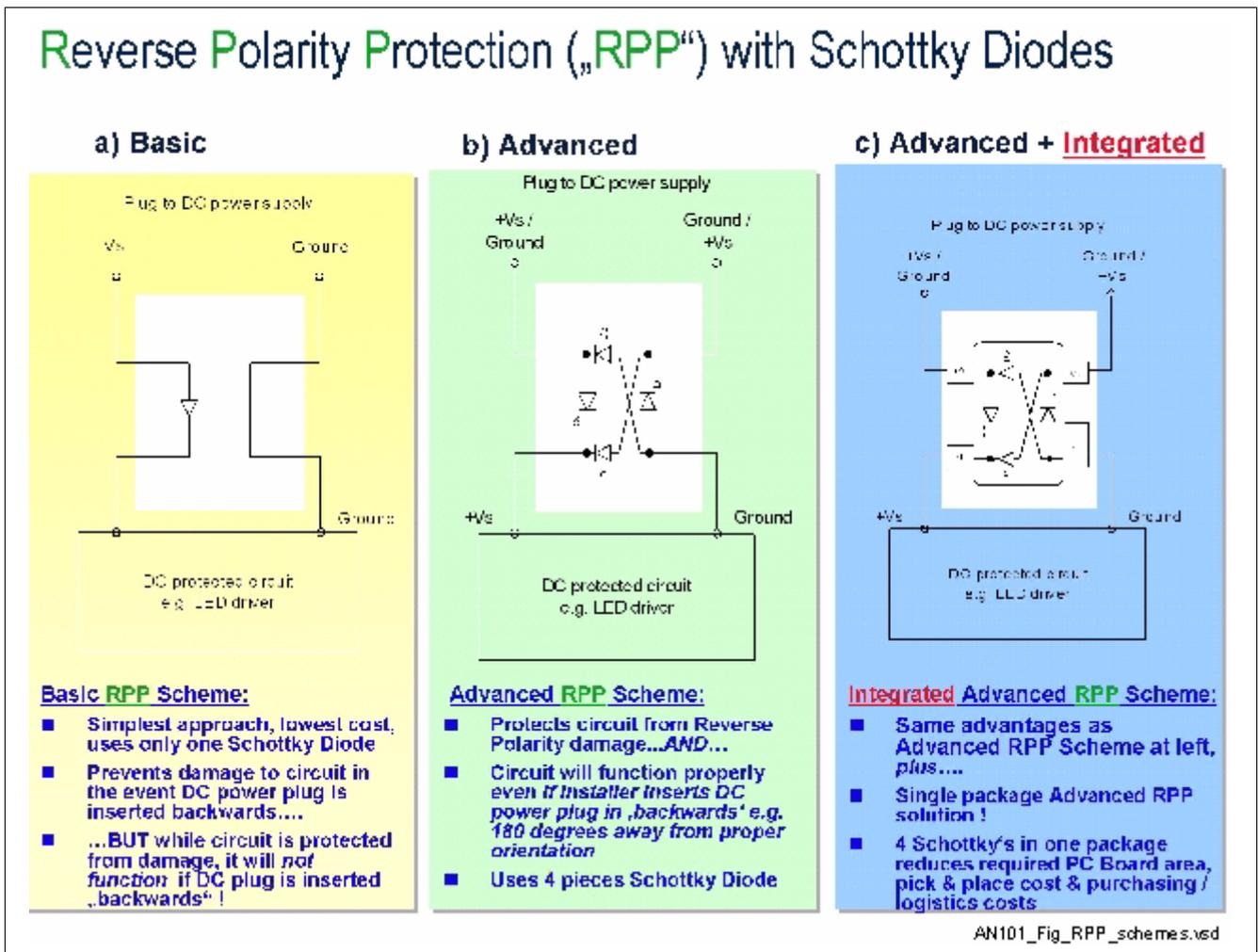
Figure 20 Three possible Reverse Polarity Protection (RPP) Schemes using Schottky Diodes
