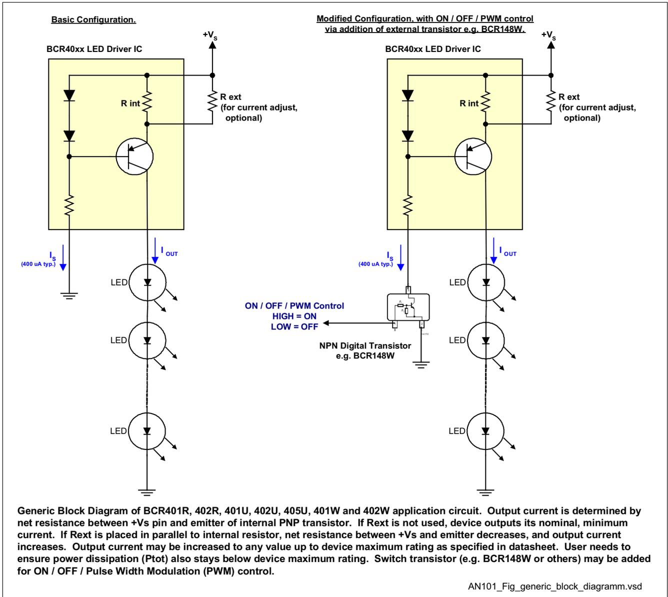
**Figure 5** Generic Block Diagram & Application Circuit, Stand-Alone LED Driver (10 - 65 mA current range). Circuit on right has added an external switching transistor to enable ON / OFF and Pulse Width Modulation (PWM) for dimming function. Optional Reverse Polarity Protection (RPP) may be added by placing a Schottky diode between  $+V_s$  and the LED Driver IC
