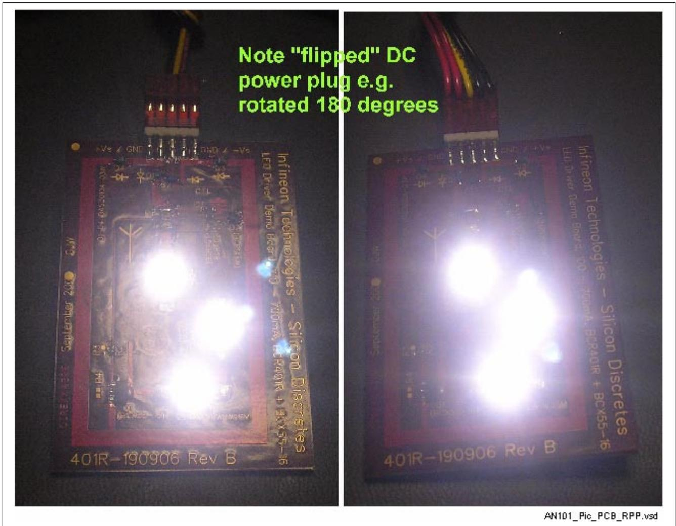
Figure 14 Photo of PCB showing RPP scheme in operation
