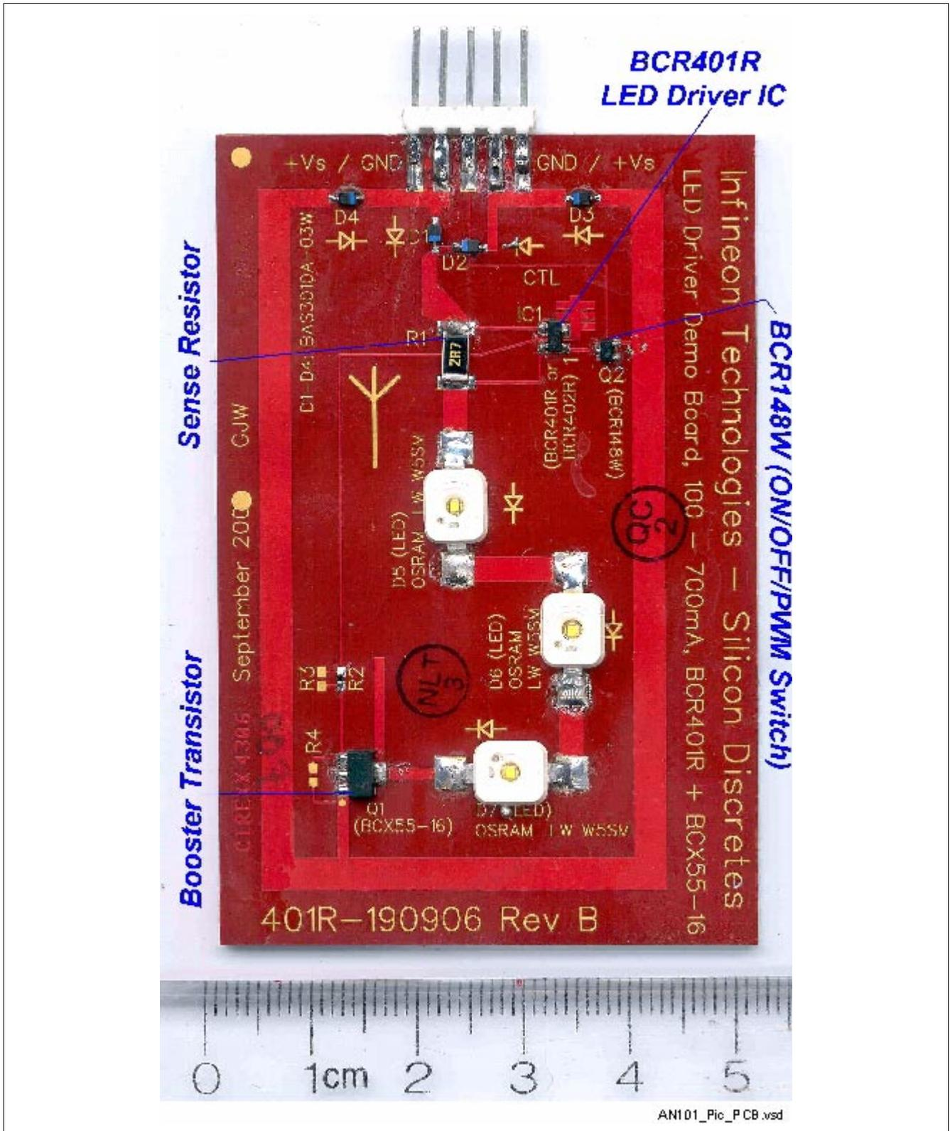
Figure 12 Photograph of Application Circuit
