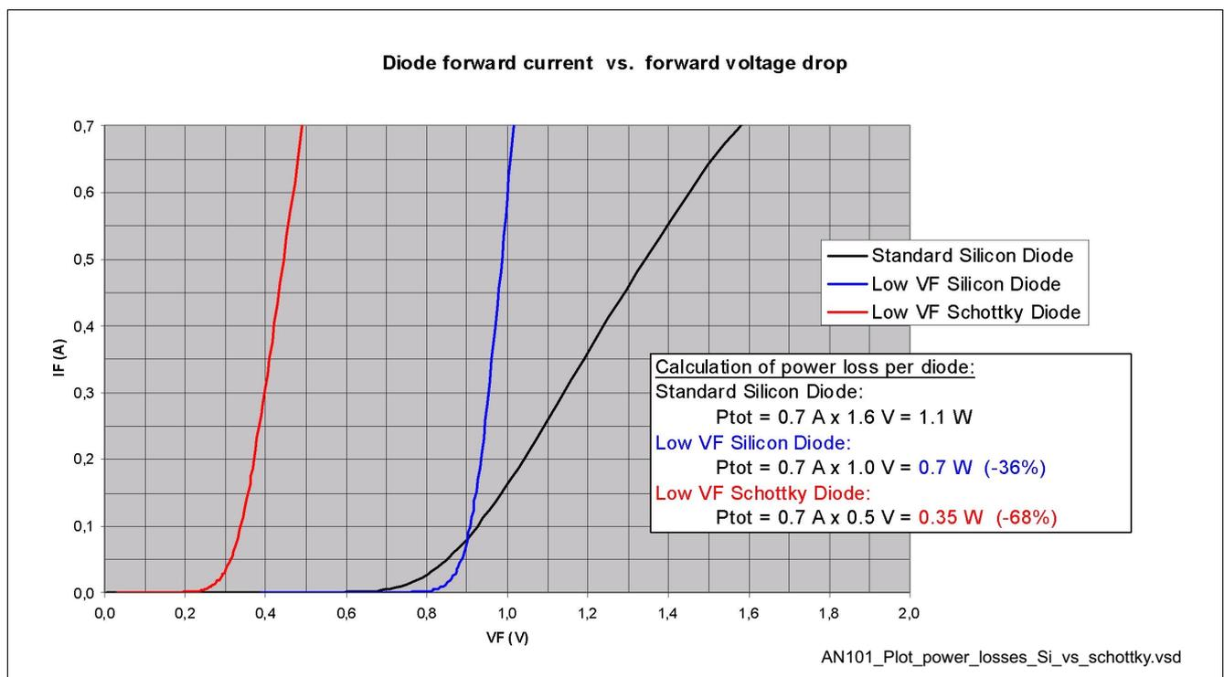
**Figure 19 Power Losses in Silicon versus Schottky Diode Types**
