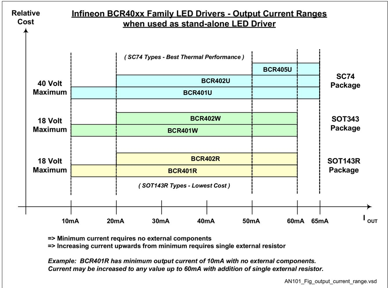
**Figure 4** Output current ranges for the standard LED Driver types. Bare device outputs nominal, minimum current with no external elements; current may be increased upwards from minimum value by addition of one external resistor. SOT143R packaged-devices are generally lowest in cost; SC74 packaged devices have best thermal performance
