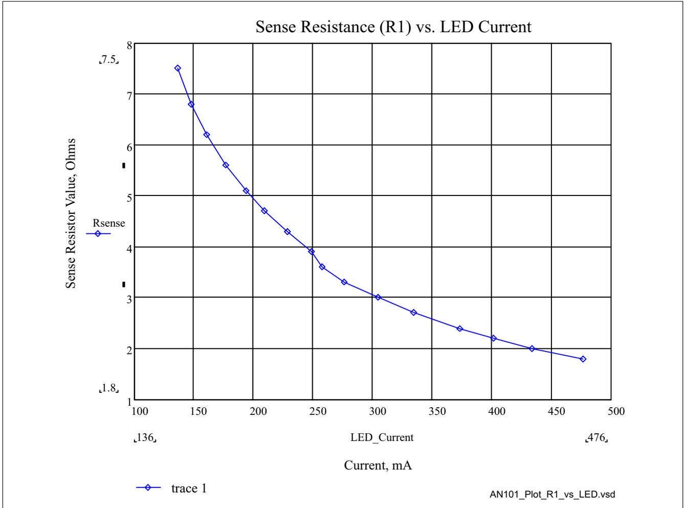
Figure 13 Sense Resistor Value (R1) vs. LED current
