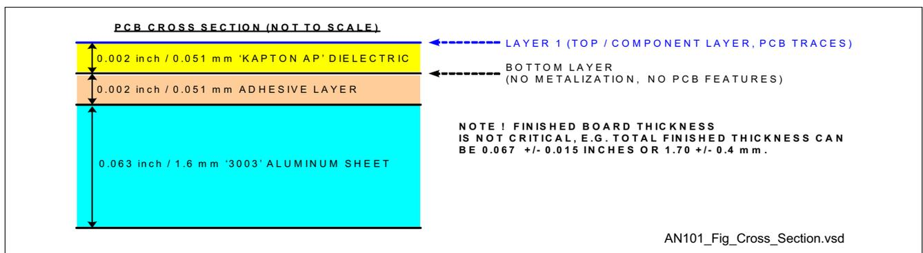
Figure 10 Cross Section Diagram of metal-clad PCB
