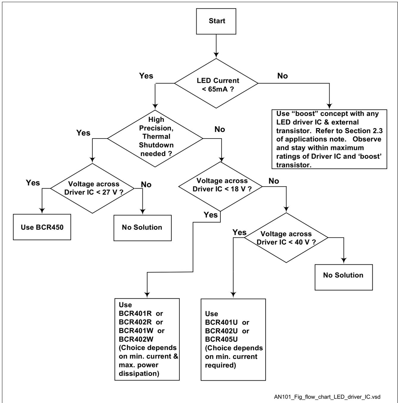
Figure 6 Flow Chart to aid in selection of the appropriate LED Driver IC
