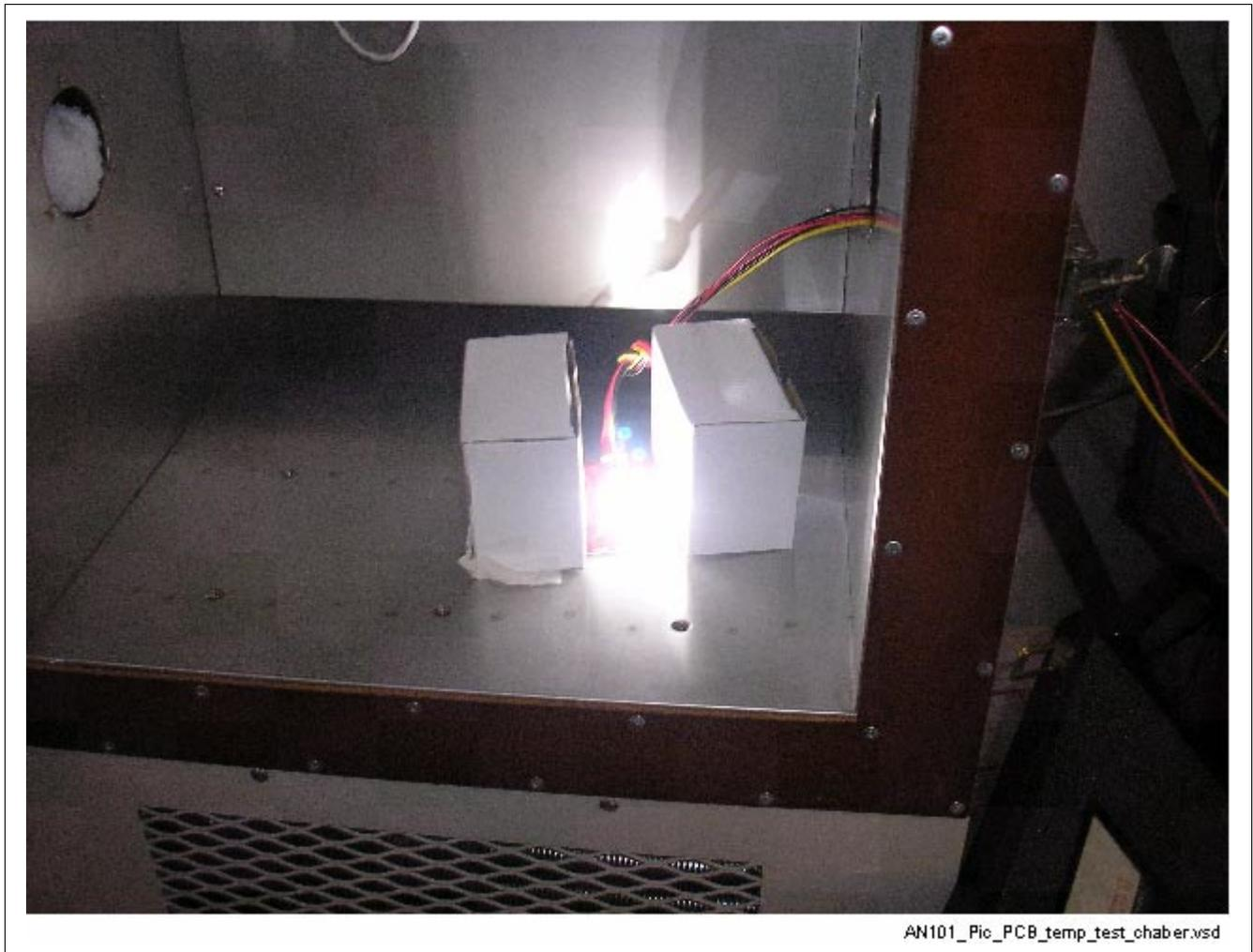
**Figure 15** Photo of PCB Assembly in Temperature Test Chamber
