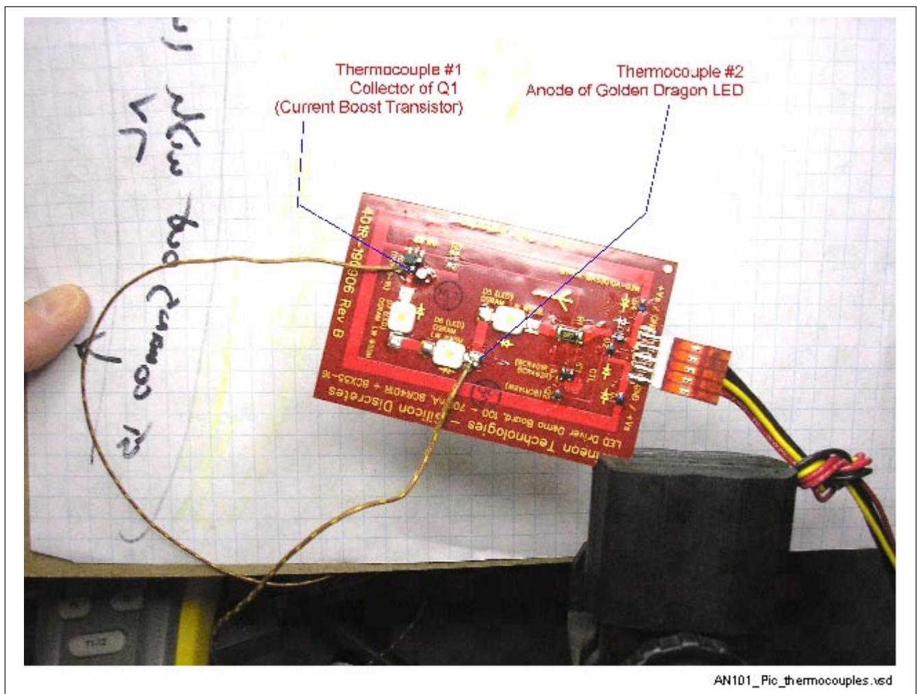
Figure 18 Photograph of locations of Thermocouples used in thermal resistance measurement
