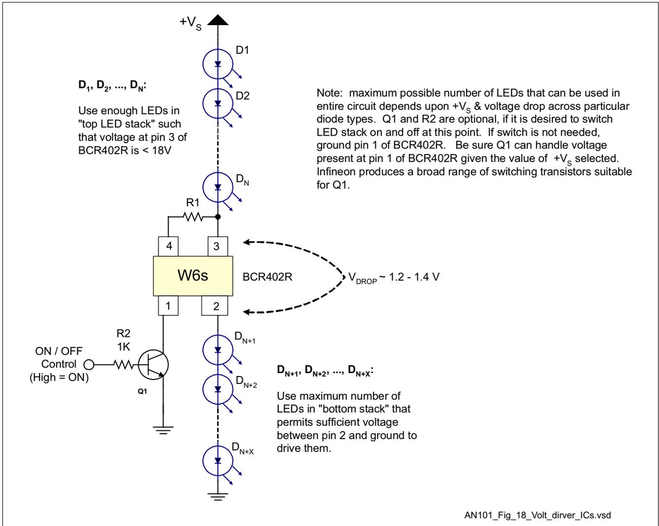
**Figure 8** Operation of 18 Volt-rated LED Driver ICs (BCR401R / 402R / 401W / 402W) at "high" power supply voltages  $> 18 V$ . Additional LEDs are inserted between the power supply voltage and the LED driver, to reduce voltage seen by the LED driver IC to a safe level,  $< 18 V$
