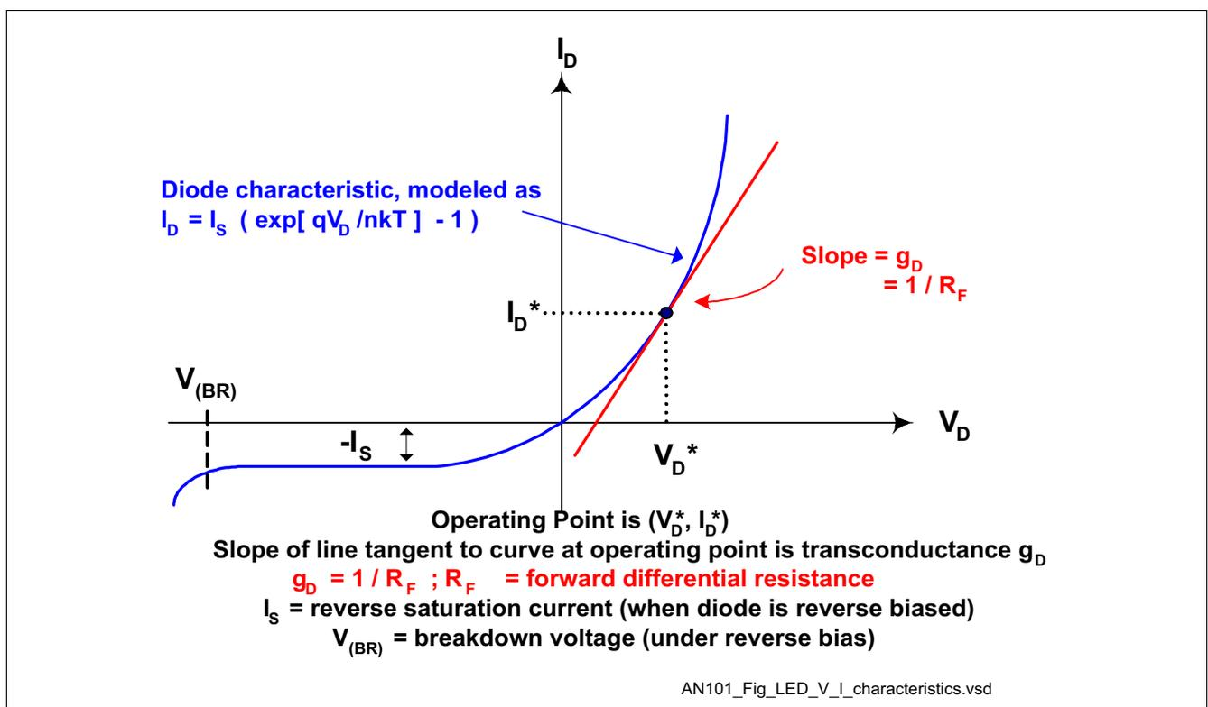
**Figure 2** LEDs, like other diodes, have an exponential voltage - current characteristic. Small changes in voltage across the LED can result in large changes in LED current
