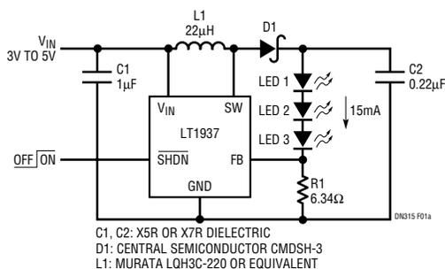
**Figure 1. Li-Ion Powered Driver for Three White LEDs**
