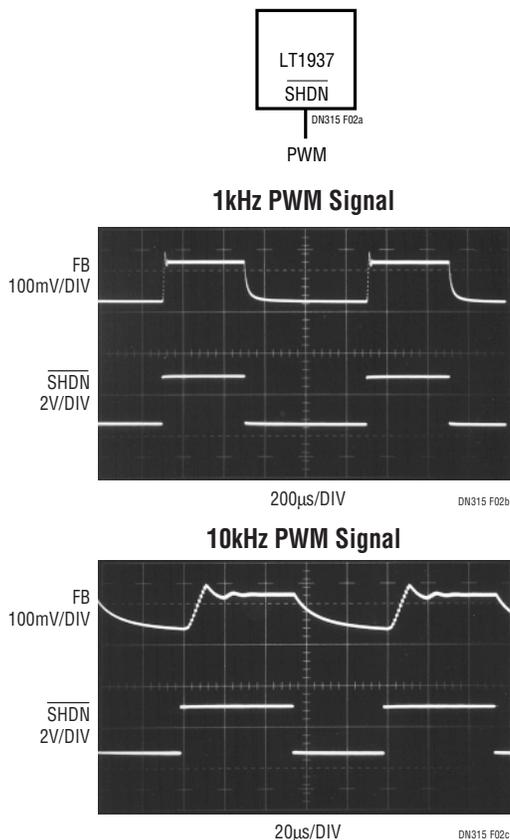
**Figure 2. PWM Dimming Control Using the SHDN Pin**
