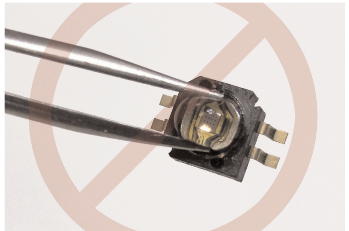
Figure 3. Incorrect handling - do not grip the lens.
