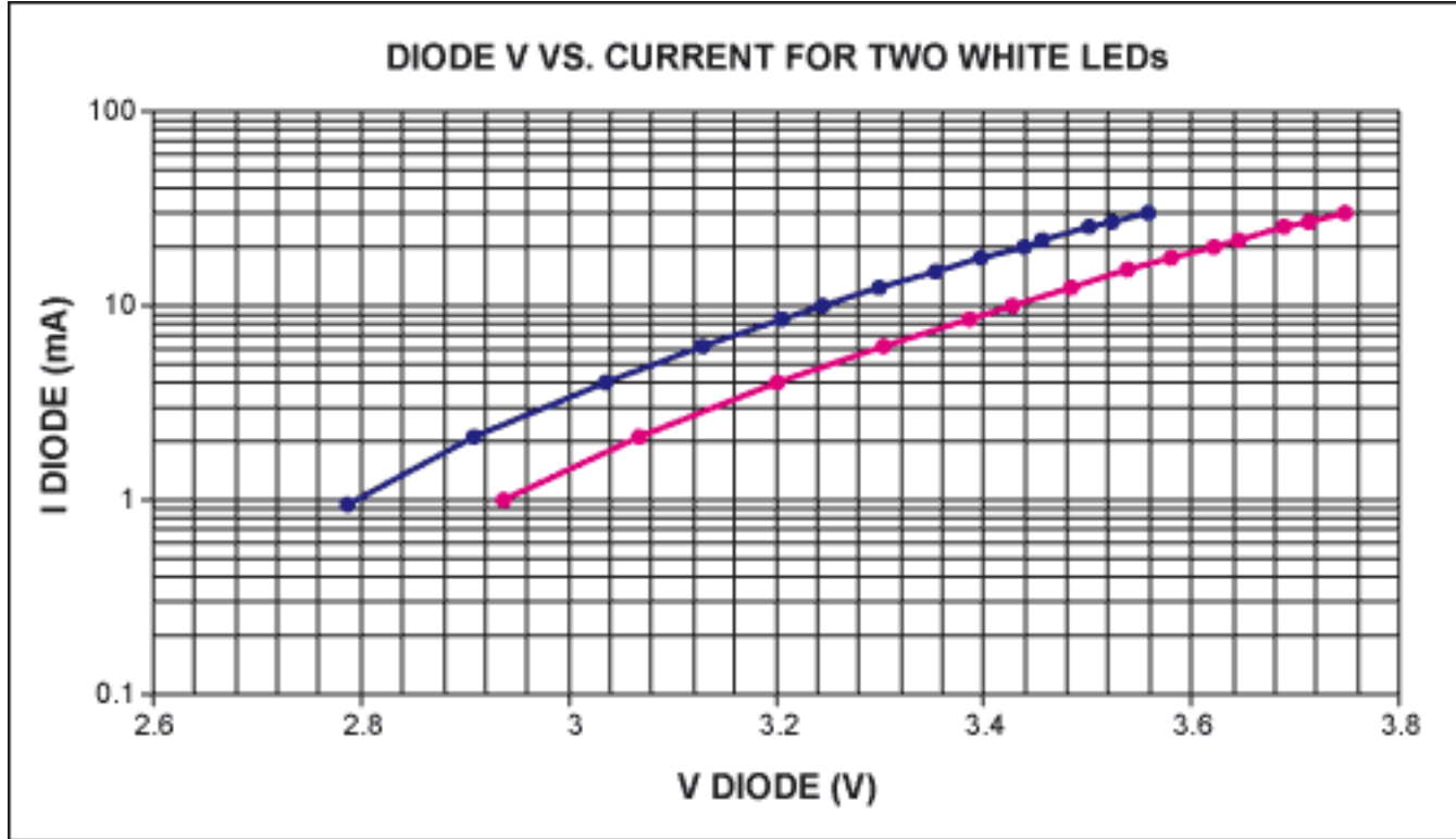
Figure 9A. The I-V curves for two white LEDs taken from a typical handheld device.
