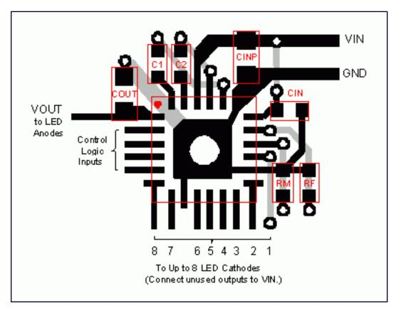
Observe the following guidelines when laying out PCB artwork for the MAX1576 white-LED charge pump:
