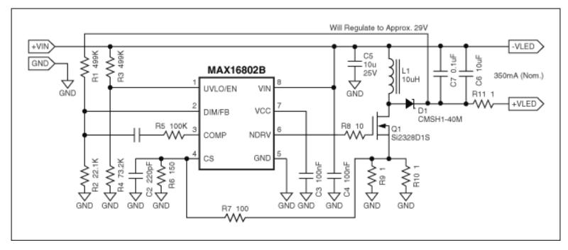
$\textbf{Caution:} \ \, \text{Avoid applying power to the circuit with the } + \text{$V_{\text{LED}}$ and $-$V_{\text{LED}}$ terminals not connected to an LED.}$
