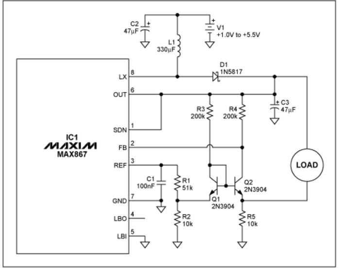
Figure 1. A low-cost feedback network (Q1, Q2, and associated resistors) improves the efficiency of this switchmode current source by a factor of six.
