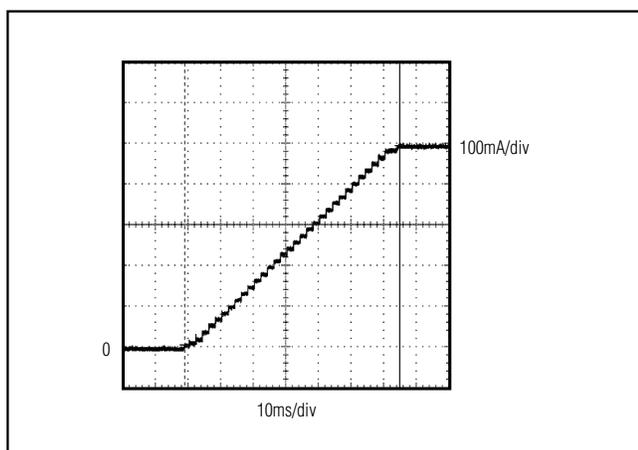
Figure 4. Typical Current Soft-Start During Initial Startup
