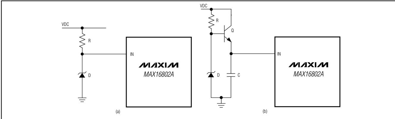
Figure 2. (a) Resistor-Zener and (b) Transistor-Zener-Resistor Bias Arrangements
