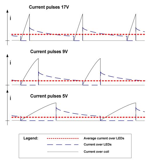
As seen in the figure: the longer time it takes to charge the coil, as lower will be the average current through the diodes in the voltage step up chain.
