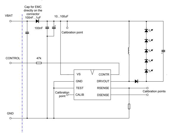
**Warning:** If the LED chain is broken (open connection), circuit will continue pumping up the voltage until the capacitor or the diode inline with LED diodes will break down. This will also put the MLX10801 into a situation outside its specified functionality. The resulting damage depends on the size of the coil. This can be eliminated with a zener diode parallel to the capacitor.
