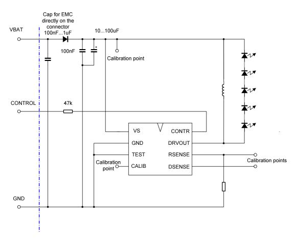
The fly back diode is needed in this circuit now only, if high supply voltages can be expected. This circuit handles VBAT voltages from 5V to (28V - n(Diode voltage)); n = number of diodes in serie. The voltage on the DRVOUT pin should never exceed 28V.
