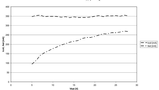
Coil/LED Current vs. Supply Voltage
