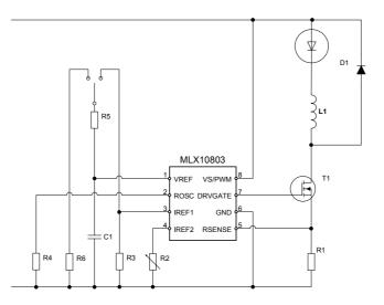
If both automatic up and down dimming is desired, the circuit above can be used. Notice; in case of down dimming in this case the circuit is still attached to the supply. If a real off-function for the down dimming is wanted, it must be combined with some kind of energy storage for the down dimming period.
