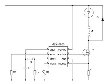
The analog dimming used in example 4.1 can also used to create an automatic slow increase of the light level when switching on power to the LED driver circuit above. The rise time is defined by the combination of R3, R5 an C1.
