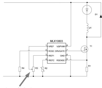
Potentiometer for dimming
