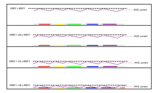
Note that the regulation does not go into discontinuous regulation mode until very low values on VREF, now when using small ripple regulation.
