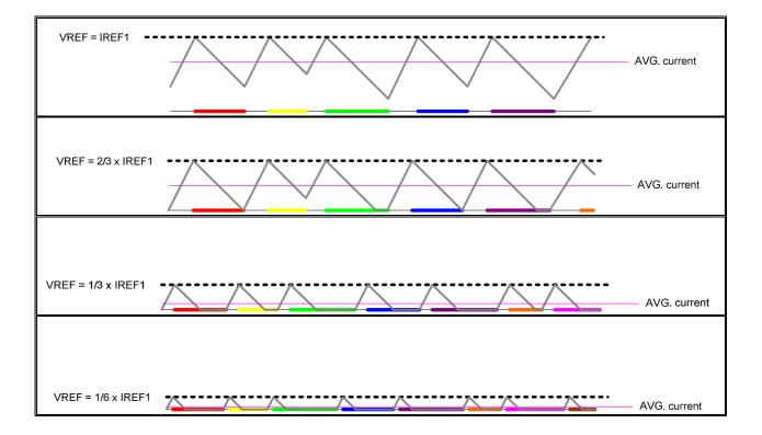
Note that the regulation goes quite quickly into discontinuous regulation mode when using large ripple regulation. It is not a problem but the linearity of the regulated current suffers.
