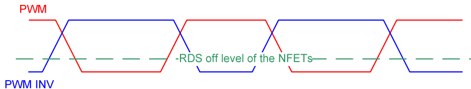
Examples of suitable PWM signal and its inverse
