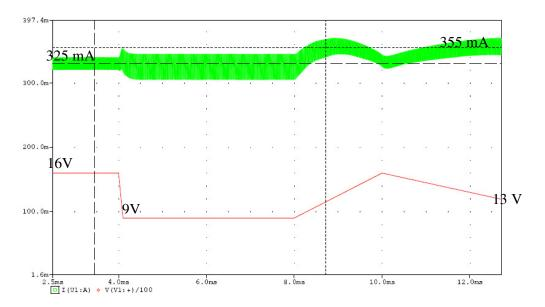
LED current(green) varies+/- 3.5% as a function of VS 355mA @13V, 330mA @9V and @16V
