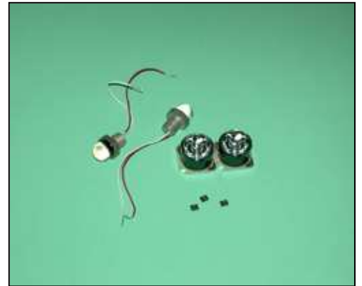
Figure 3: The MLX10801 (front) can be used as a driver for high-performance visible-light and infrared LEDs
