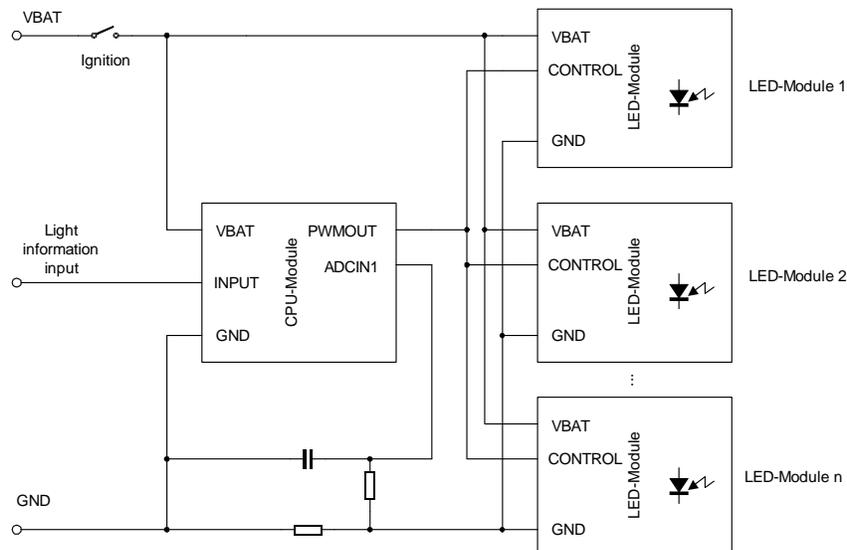
The ground shift of the LED modules due to the sense resistor is not a problem, in the LED-Modules is an internal protection resistor on the LED-Module pin CONTR.
