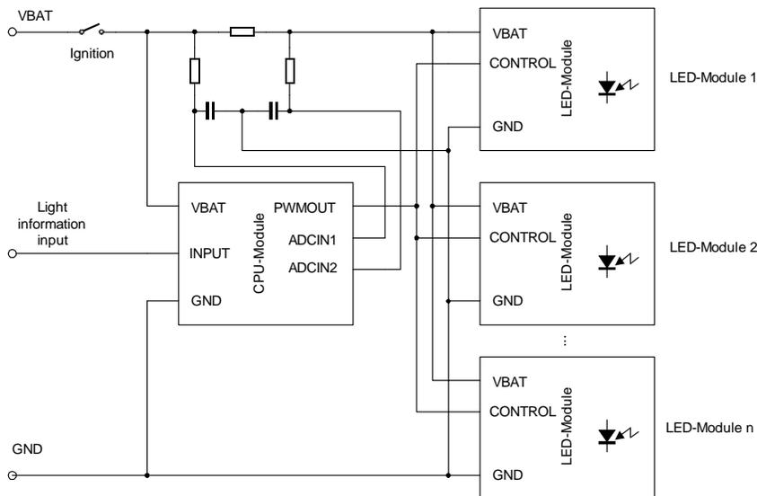
The current measurement in the supply could be changed to the current measurement in the ground lines of the LED modules. Just one ADC channel is needed as the next figure shows,
